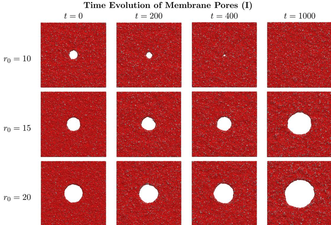
Figure 2: Rendered images of pores of three different initial sizes (rows). Four images throughout the simulation are shown, progressing from left to right. Pores shrink or grow exponentially depending on the initial pore radius.
