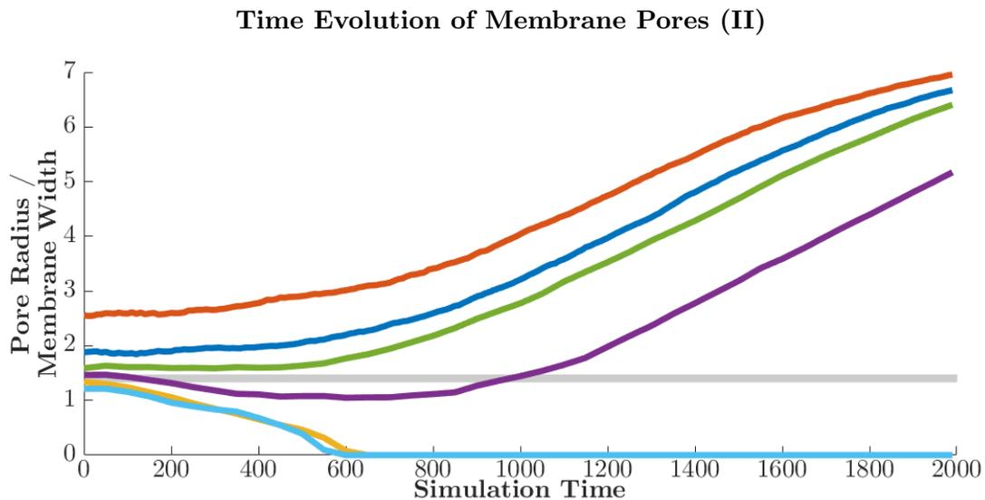
Figure 3: Membrane pore size over time as calculated by Eq. (2). Size ( $y$  axis) is shown in units of the average membrane width,  $h = 7.98$ . Several initial sizes are shown, ranging from  $r_0/h = 1.21$  (bottom) to  $r_0/h = 2.56$  (top). The shaded region denotes possible values of the critical ratio  $r_c/h$  below which pores seal –  $1.34 < r_c/h < 1.47$ .
