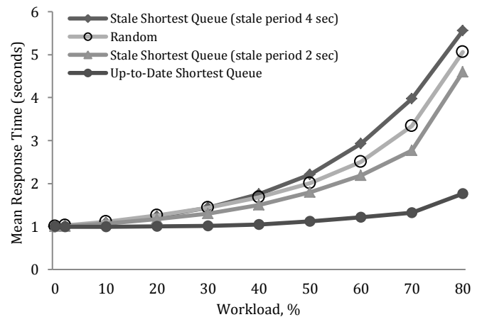
Figure 3. Comparison of the mean response time of the Shortest Queue balancing strategy with stale information to Random and Up-to-Date Shortest Queue strategies. Two different stale periods are shown.
