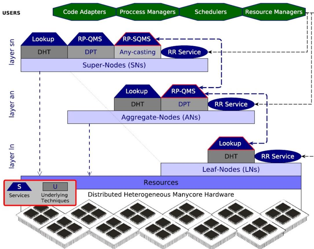
Figure 2: Resource Discovery System Architecture.
