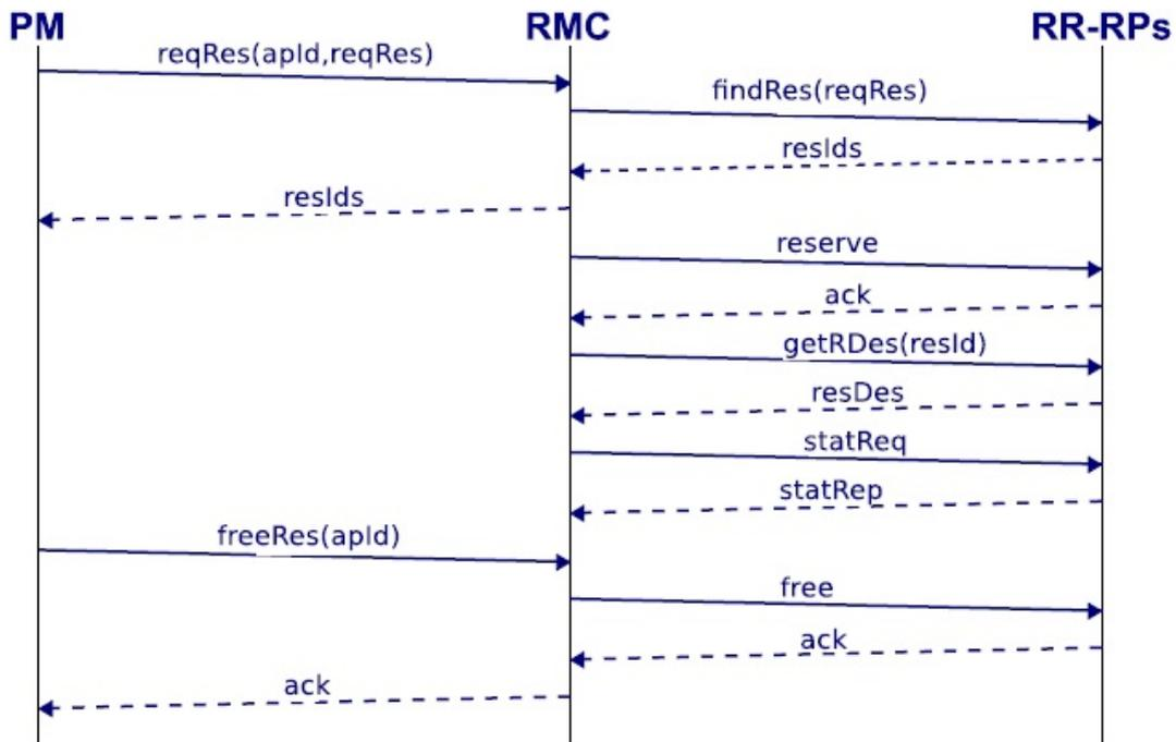
Figure 6: Message sequences for the interactions between RR, RP and RMC.
