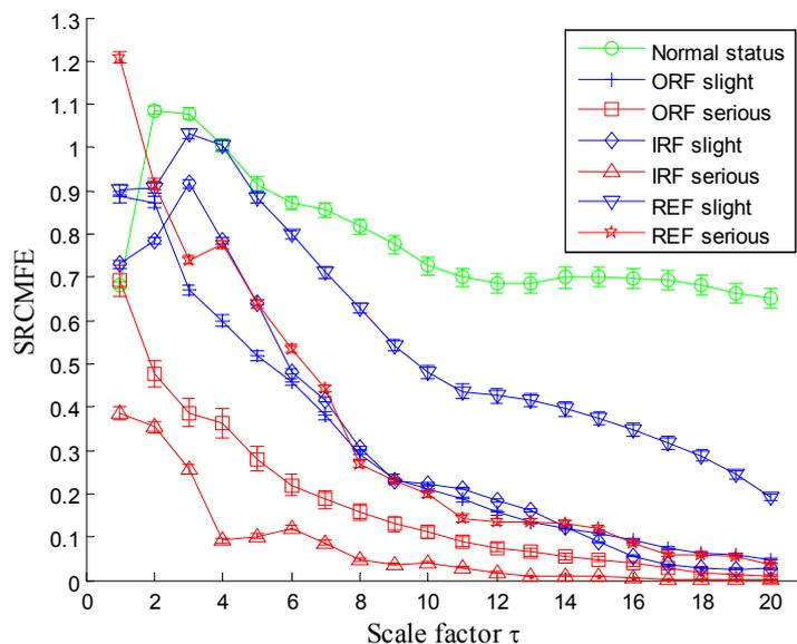
Fig.8 SRCMFE over 20 scales of the corresponding vibration signals
