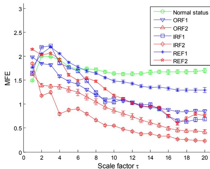
Fig.11 MFE over 20 scales of the corresponding vibration signals
