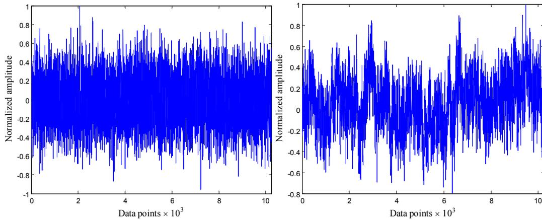
(a) Waveforms of Gaussian white noise (b) Waveforms of Gaussian 1/f noise
