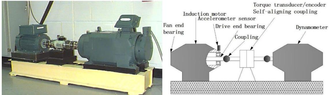
Fig.6 The rolling bearing experiment system and its sketch
