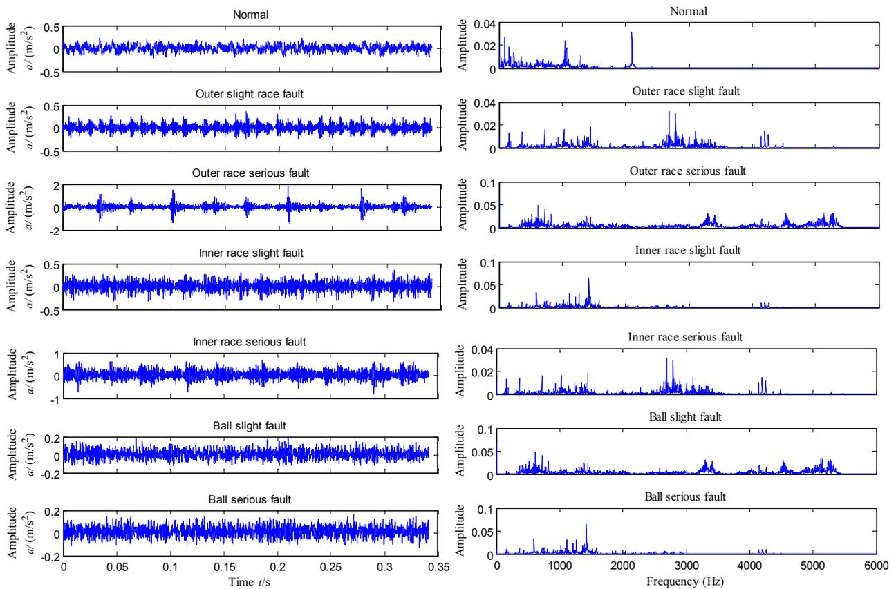
(a) Time waveform of vibration signals
