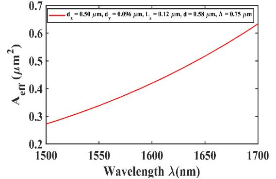
Fig. 3 Effective area vs. wavelength of the proposed HNL-PCF with parameters  $\Lambda = 0.75 \mu\text{m}$ ,  $d = 0.58 \mu\text{m}$ ,  $d_x = 0.5 \mu\text{m}$ ,  $d_y = 0.096 \mu\text{m}$  and  $L_s = 0.12 \mu\text{m}$ .
