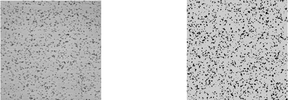
Figure 2: The deposition surface of the Impact-R device after 300 seconds (left) and the corresponding results of the deposition in the mathematical model (right). Black dots represent the deposited platelets that are grouped in clusters.
