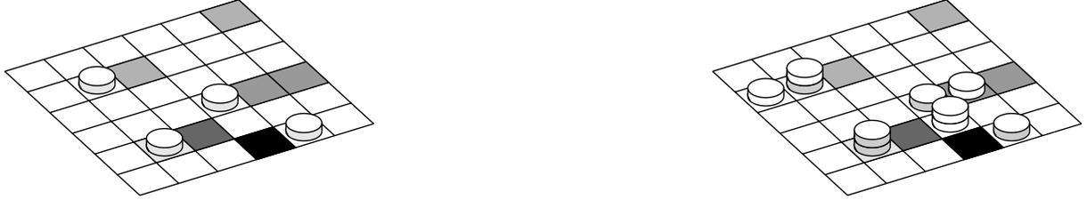
Figure 1: Sketch of the deposition substrate, discretized in cells of area equal to the surface of a platelet.
