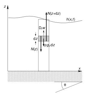
Fig. 2. Schematic representation of an infinitesimally thin column of an avalanche on a plane inclined at an angle  $\theta$  and an infinitesimal control volume within that column. Only the forces relevant for the bed-normal motion are indicated.
