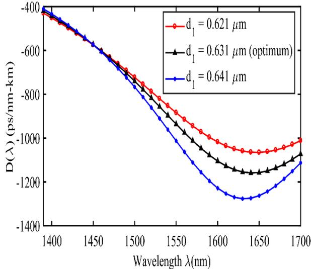
Fig. 4. Chromatic dispersion of the signified DC-PCF as function of wavelength with the parameter  $d_1$  taken as  $0.621 \mu\text{m}$ ,  $0.631 \mu\text{m}$  and  $0.641 \mu\text{m}$  keeping  $d_2$ ,  $\Lambda_2$  and  $\Lambda_1$  unaltered.
