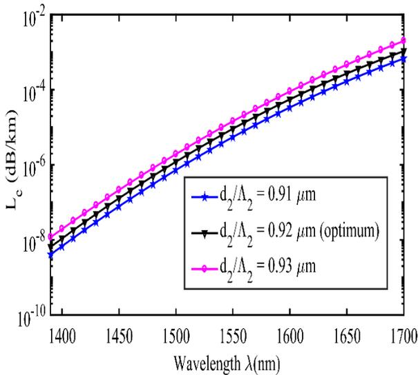
Fig. 9. Confinement loss vs. wavelength for the changing  $d_2/\Lambda_2$  from 0.91  $\mu\text{m}$  to 0.93  $\mu\text{m}$  keeping other parameters unaltered.
