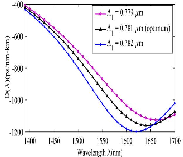
Fig. 6. Chromatic dispersion of the denoted DC-PCF as function of wavelength with the parameter  $\Lambda_1$  taken as  $0.779 \mu\text{m}$ ,  $0.781 \mu\text{m}$  and  $0.782 \mu\text{m}$  keeping  $d_2$ ,  $\Lambda_2$  and  $d_1$  unchanged.
