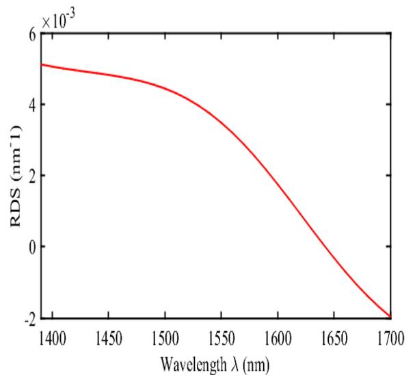
Fig. 11. RDS of the proposed DC-PCF vs. wavelength for the optimum parameters  $d_1$ ,  $\Lambda_1$ ,  $d_2$  and  $\Lambda_2$ .
