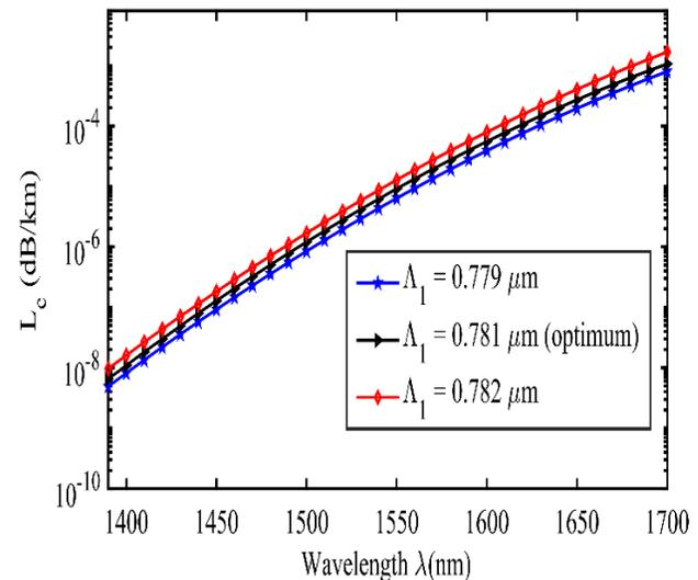
Fig. 7. Confinement Loss of the proposed DC-PCF as function of wavelength with the parameter  $\Lambda_1$  taken as  $0.779 \mu\text{m}$ ,  $0.781 \mu\text{m}$  and  $0.782 \mu\text{m}$  keeping  $d_2$ ,  $\Lambda_2$  and  $d_1$  untouched.
