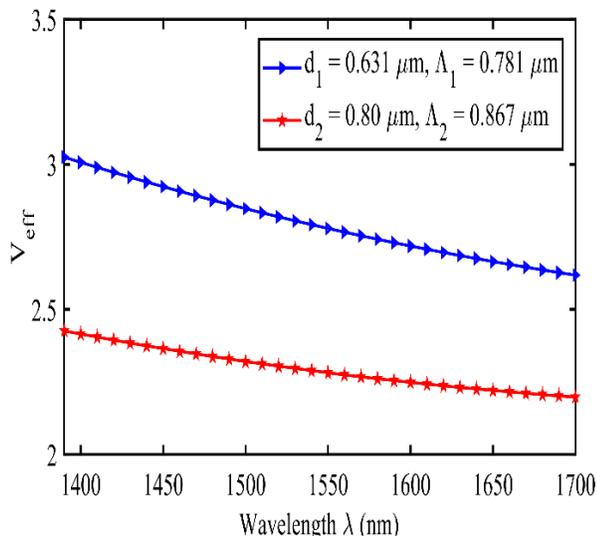
Fig. 12. V-parameter of the proposed DC-PCF as a function of wavelength for the inner and outer cladding with the optimum geometric entities.
