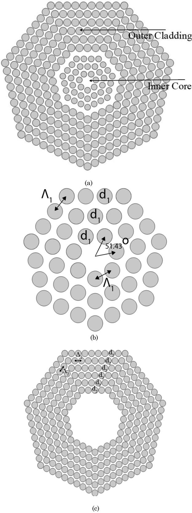
Fig. 1. Transverse cross section of the suggested DC-PCF with the optimum parameters  $d_1$ ,  $d_2$ ,  $\Lambda_1$  and  $\Lambda_2$ . (a) Full cross sectional view of DC-PCF, Cross sectional view of (b) magnified core (c) Cladding
