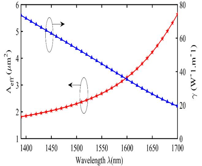
Fig. 10. Nonlinear co-efficient and effective area as a function of wavelength for the optimum parameter of the Proposed DC-PCF.
