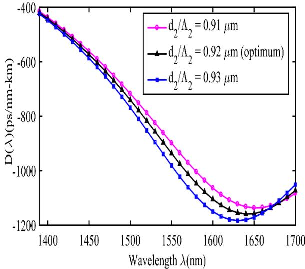
Fig. 8. The proposed DC-PCF's chromatic dispersion as a function of wavelength changing  $d_2/\Lambda_2$  from 0.91  $\mu\text{m}$  to 0.93  $\mu\text{m}$  keeping other parameters unaltered.
