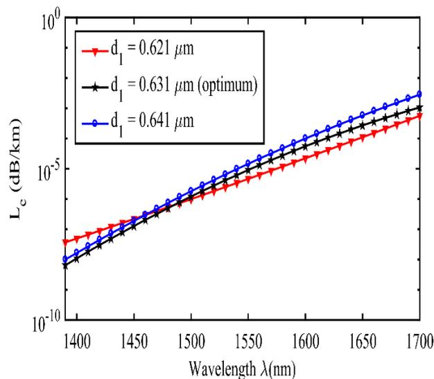
Fig. 5. Confinement loss vs. wavelength with parameter  $d_1$  taken as  $0.621 \mu\text{m}$ ,  $0.631 \mu\text{m}$  and  $0.641 \mu\text{m}$  keeping  $d_2$ ,  $\Lambda_2$  and  $\Lambda_1$  unchanged.
