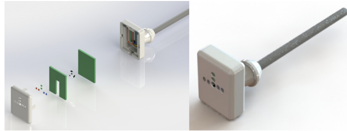
Fig 1. Prototype of the sensor probe. (A) Exploded perspective drawing of optoelectronic components fitting in the cover probe. (B) 3D illustration of the second version of the sensor module. Note: Exact positions between the LEDs and photodiode, in the middle of the sensor are: Red 1 = 3.3 mm; Red 2 = 6.5 mm; Green 1 = 4.0 mm; Green 2 = 7.2 mm; Blue 1 = 3.3 mm; Blue 2 = 6.5 mm.
