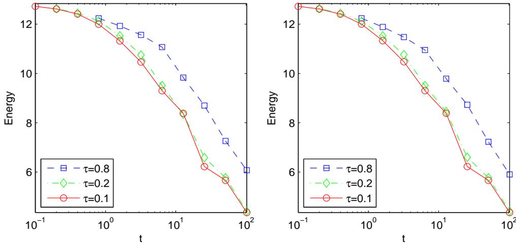
**Fig. 2** The discrete energy dissipation of the two schemes solving the Cahn-Hilliard equation with initial value  $\phi_1$ , and relaxation parameter  $\gamma = 0.0025$ . Stability constant  $A = 0.25, B = 20$  are used. Left) result of SL-CN scheme; Right) result of SL-BDF2 scheme.
