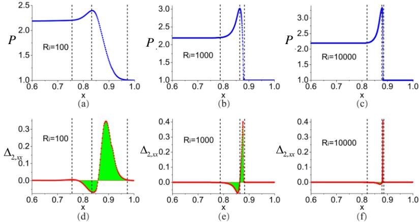
**Figure 2.** Profiles of physical quantities for different relaxation times. (a)-(c) are for the pressure  $P$ . (d)-(f) are for the corresponding non-equilibrium quantities  $\Delta_{2,xx}$  ( From Ref. [22] with permission ).
