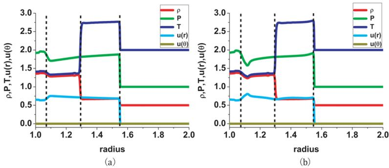
**Figure 6.** Profiles of physical quantities in the process of shock wave passing outwards from the heavy medium to the light one. (a) Without initial perturbations at the interface. (b) With initial sinusoidal perturbation at the interface (From Ref. [25] with permission).
