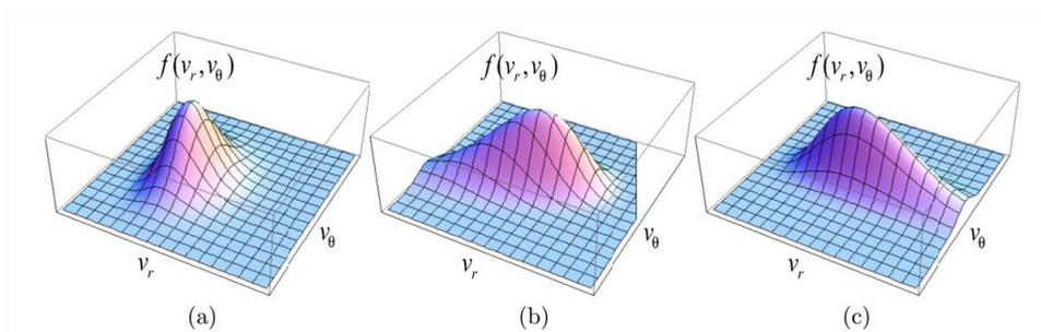
**Figure 7.** Sketches of the actual distribution functions in velocity space  $(v_r, v_\theta)$ . Panels (a)-(c) show the recovered distribution functions at the rarefaction wave, the material interface, and the shock wave, respectively (From Ref. [25] with permission).
