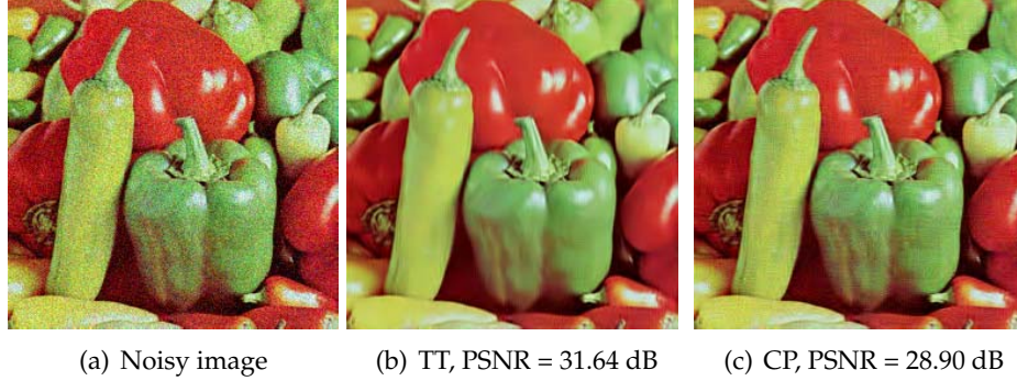
Figure 1.8: Tensor based image reconstruction in Example 8. The Pepper image with added noise at 10 dB SNR (left), and the images reconstructed using the TT (middle) and CP (right) decompositions.
