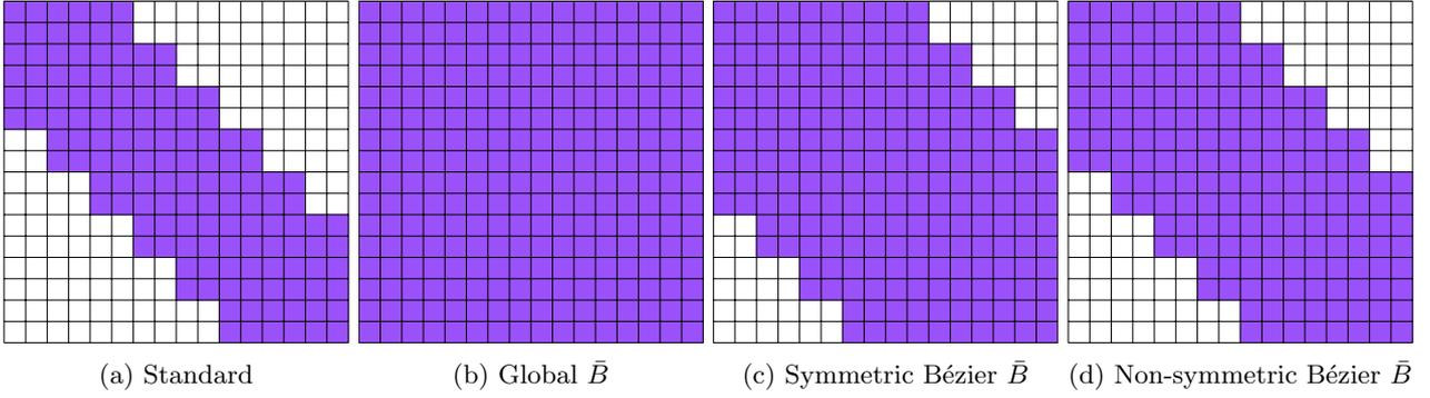
Figure 6: Illustrations of the structure of  $2^{nd}$  order Timoshenko beam stiffness matrices for (a) a standard displacement method, (b) a global  $\bar{B}$  method, (c) a symmetric Bézier  $\bar{B}$  method and (d) a non-symmetric Bézier  $\bar{B}$  method.
