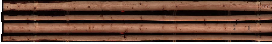
FIG 1. Sample lumber used in the real data analysis. Four sides of the boards with the wide surfaces shown on the first and the third rows and the narrow surfaces shown on the second and the last rows.
