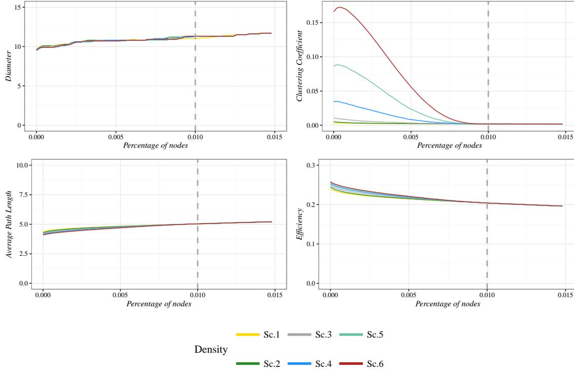
Figure 4: Resilience for simultaneous attack simulations with progressive manipulation of number of links in the network core; magnification of the area of Figure 3 in which lays the rich-club. The dashed line is placed in correspondence to the rich-club size. All are results averaged over 10 instances.
