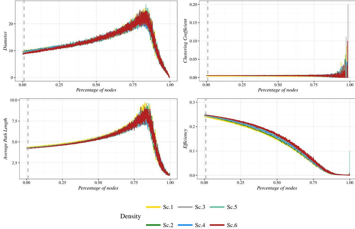
Figure 8: Resilience for simultaneous error simulations with progressive manipulation of the number of links in the network periphery. The dashed line is placed in correspondence to the rich-club size. All results are averaged over 10 instances.
