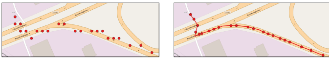
Fig. 4: OpenStreetMap routing tool is applied to map match time-stamped sequence of latitude/longitude pairs (left) to most likely road-based routes (right).
