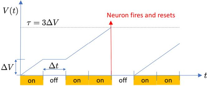
Fig. 1. Illustration of the neuron model with integrate-and-fire. In this example,  $n_{\min} = 3$ , i.e., spikes must be separated by at least  $3\Delta t$ . In each interval when the light source is on, the voltage increases by  $\Delta V$ . Once the threshold  $\tau = 3\Delta V$  is reached, the neuron fires and resets to  $V(t) = 0$ .
