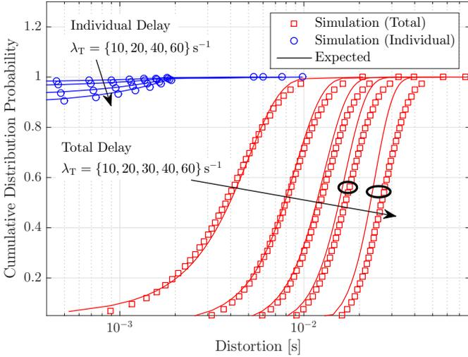
Fig. 4. Distribution of the delay distortion  $\bar{d}(\vec{u}, \vec{v})$  for different values of target generation rate  $\lambda_T$ . The target sequence has a length of  $M = 200$  spikes, and the minimum time that we must wait before generating another spike in  $\vec{v}$  is  $t_{\min} = 2$  ms.
