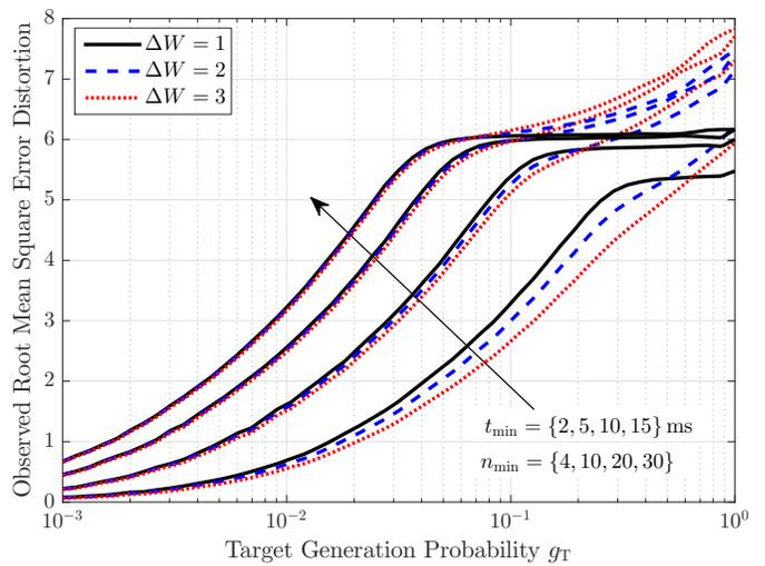
Fig. 10. Average observed (i.e., simulated) RMSE  $\bar{d}(\vec{u}, \vec{v})$  as a function of the target firing probability  $g_T$  in each time slot. We vary the number  $n_{\min}$  of slots that it takes to charge the neuron, and consider metric kernels with lengths  $\Delta W \in \{1, 2, 3\}$  slots. The minimum wait times  $t_{\min} = \{2, 5, 10, 15\}$  ms correspond to  $n_{\min} = \{4, 10, 20, 30\}$  slots.
