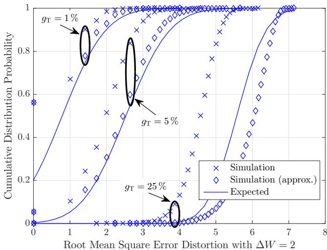
Fig. 8. Distribution of RMSE  $d(\vec{u}, \vec{v})$  when the metric kernel has length  $\Delta W = 2$ . Target firing probabilities of  $g_T = \{1, 5, 25\}\%$  are considered. The target sequence has a length of  $M = 20$  spikes, and we are constrained by a charging time of  $n_{\min} = 4$  slots when generating spikes in  $\vec{v}$ .
