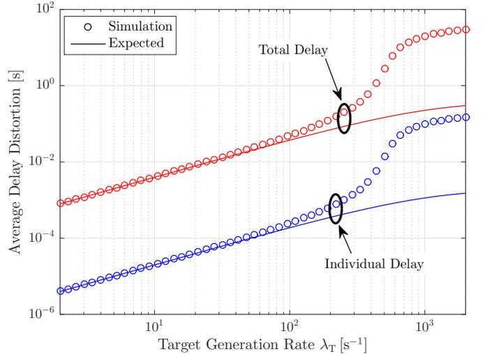
Fig. 3. Average delay distortion  $\bar{d}(\vec{u}, \vec{v})$  as a function of the target generation rate  $\lambda_T$ . The target sequence has a length of  $M = 200$  spikes, and the minimum time that we must wait before generating another spike in  $\vec{v}$  is  $t_{\min} = 2$  ms. The total (cumulative) delay for a given sequence is the sum of the individual delays.
