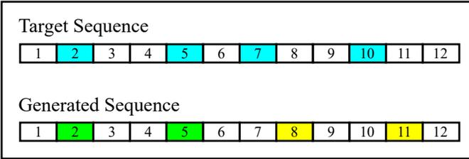
Fig. 2. Example of target sequence matching in discrete time, where the generated sequence is constrained by a charging time of  $n_{\min} = 3$  slots. Slots are labeled chronologically and colored when there is a spike at the start of the slot. The target sequence has 4 pulses (shown in blue). The generated sequence can match the first 2 pulses (green, in the 2nd and 5th slots), but the final 2 pulses (yellow, in the 8th and 11th slots) each have a delay of one slot.
