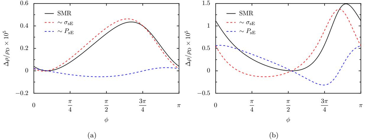
Figure 6. Ferromagnetic contribution to the SMR as function of  $\phi$  with  $\tau_s/\tau_{\text{DP}} = 10$  and  $g_r^{\uparrow\downarrow}\alpha\tau_{\text{DP}}/\hbar = 10$  for  $L = 10l_{\text{DP}}$ , (a), and  $L = l_{\text{DP}}$ , (b). The dashed curves represent the contributions proportional to  $\sigma_{\text{sE}}$  (red) and  $P_{\text{sE}}$  (blue), respectively. All data are normalized by  $\rho_{\text{D}} = 1/\sigma_{\text{D}}$ .
