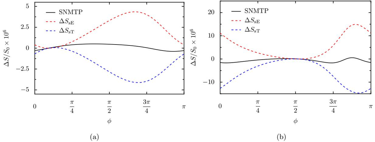
Figure 7. Ferromagnetic contribution to the SNMTP as function of  $\phi$  with  $\tau_s/\tau_{\text{DP}} = 10$  and  $g_r^{\uparrow\downarrow}\alpha\tau_{\text{DP}}/\hbar = 10$  for  $L = 10 l_{\text{DP}}$ , (a), and  $L = l_{\text{DP}}$ , (b). The dashed curves represent the electrical part (red) and the thermal part (blue), respectively.
