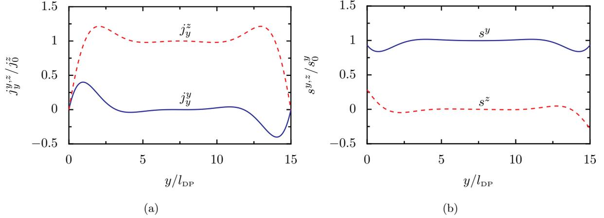
Figure 2. Spatial profile of the spin currents, (a), and the spin polarizations, (b), for symmetric boundary conditions ( $g_r^{\uparrow\downarrow} = 0$ );  $L/l_{\text{DP}} = 15$ ,  $\tau_s/\tau_{\text{DP}} = 10$ .
