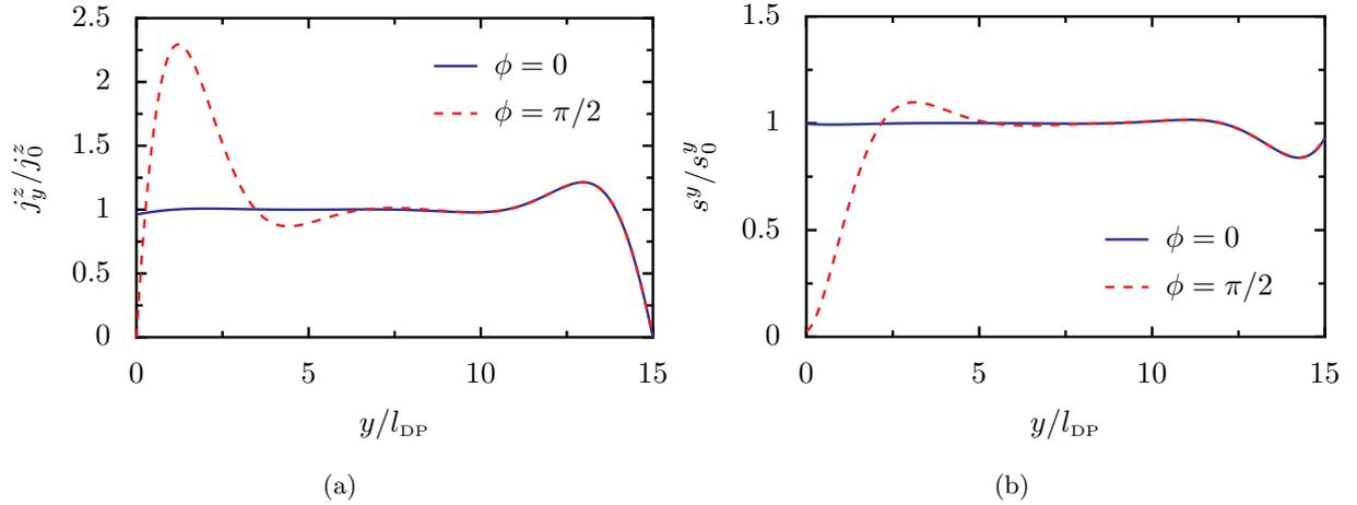
Figure 3. Spatial profile of the spin current  $j_y^z$ , (a), and the spin polarization  $s^y$ , (b), for asymmetric boundary conditions with  $g_r^{\uparrow\downarrow}\alpha\tau_{\text{DP}}/\hbar = 10$  and  $\phi = 0, \pi/2$ . The parameters  $L/l_{\text{DP}}$  and  $\tau_s/\tau_{\text{DP}}$  are the same as in Fig. 2.
