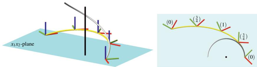
**Fig. 1** The planar motion (right) is obtained as top view of the Schoenflies motion (left). In addition we label the poses of the top view by the  $x_3$ -coordinate. In German such a map is known as "kotierte Projektion".
