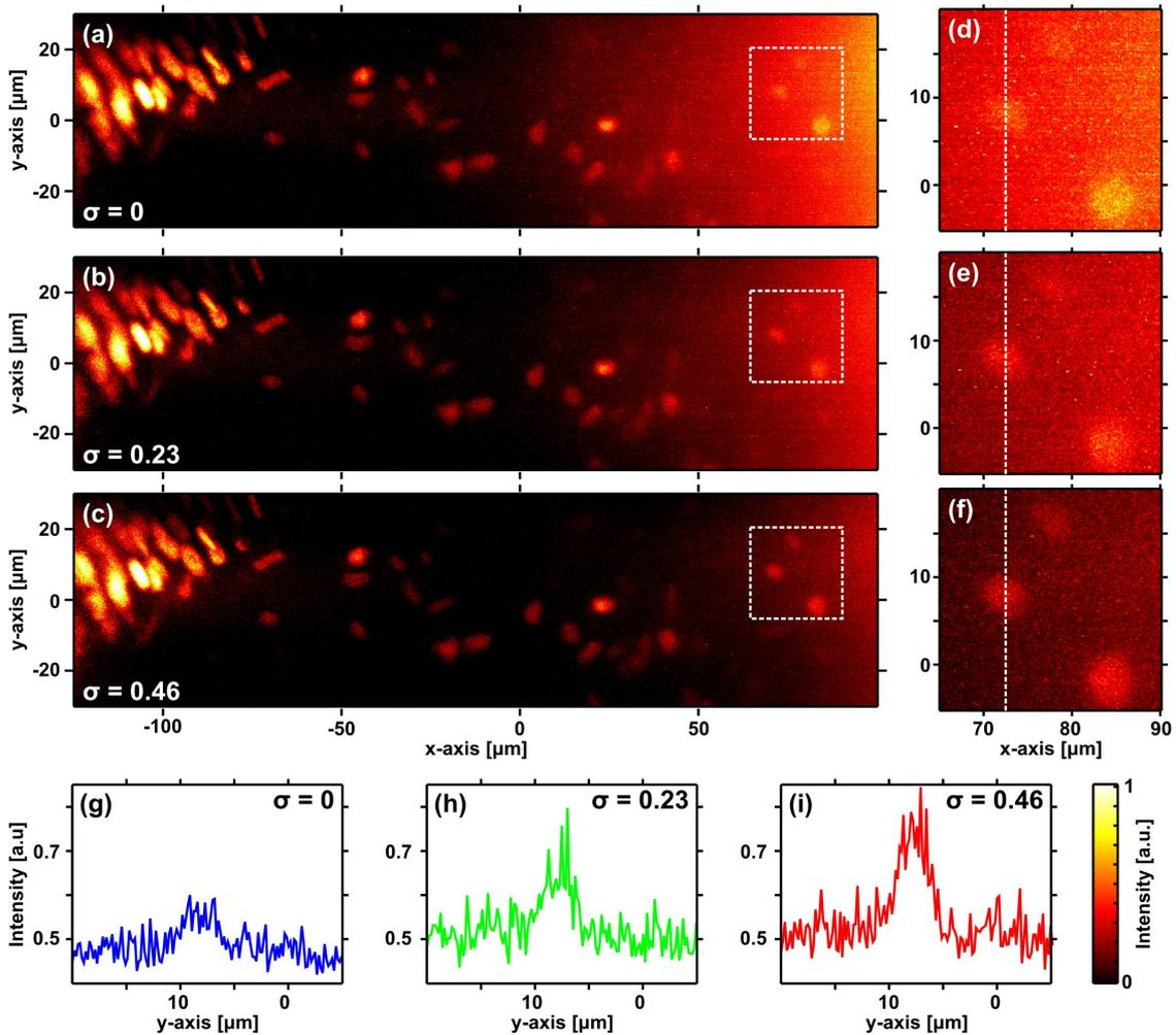
Figure 3: Maximum intensity projections of deconvolved Airy LSM images of nuclei stained with propidium iodide in the operculum of *S. lamarcki* (attenuation estimated at  $85\text{cm}^{-1}$ ) with (a) no attenuation-compensation, (b)  $\sigma = 0.23$ , (c)  $\sigma = 0.46$ . (d-f) show expanded views of the region indicated by the dashed box in (a-c). (g-i) show intensity profiles along the dashed line shown in (d-f). These datasets can be accessed at [32].
