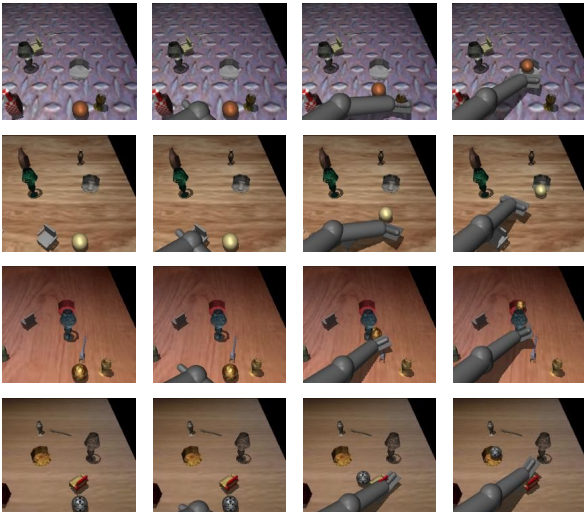
Figure 11. Some example trajectories of the striking task for from the training and testing environments. The images shown in the first row are from the training environment, while the three rows below that are examples of the test environments - with different textures, lighting conditions, and positioning of the objects.
