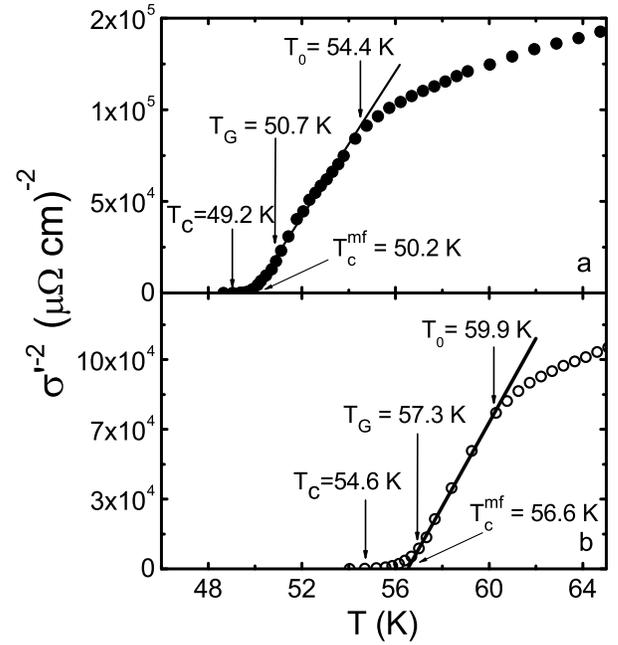
FIG. 4:  $\sigma'^{-2}$  as a function of  $T$  at  $P=0$  GPa (panel a, dots) and  $P=1.05$  GPa (panel b, circles). The straight lines follow the low  $\sigma'^{-2}(T)$  which actually corresponds to the 3D AL fluctuation region. All temperatures designated by the arrows in the figure are discussed in the text.
