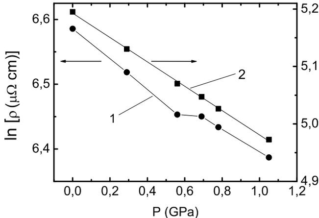
FIG. 2: Pressure dependence of  $\ln \rho$  of the  $YBa_2Cu_3O_{6.5}$  single crystal at 288 K (curve 1, dots). Solid line is guide for the eye. Squares (curve 2) represent  $\ln \rho(P)$  measured at  $T=100$  K along with the least-squares fit.
