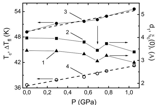
FIG. 6: Pressure dependence of  $\xi_c(0)$  (curve 1),  $d_1$  (curve 2),  $T_c$  (curve 3) and  $\Delta T_{fl}$  (curve 4). Solid lines are guides for the eye. Dashed lines are the lines of least-squares fit. Vertical arrow designates the peculiarity at  $P \approx 0.7$  GPa.
