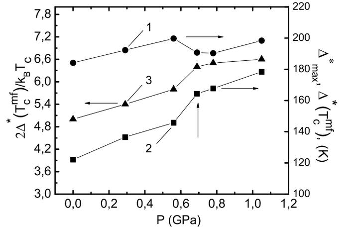
FIG. 11: Pressure dependence of  $\Delta_{max}^*$  (curve 1),  $\Delta^*(T_c^{mf})$  (curve 2) and  $D^* = 2\Delta^*(T_c^{mf})/k_B T_c$  (curve 3). Solid lines are guides for the eye. Vertical arrow marks the peculiarity at  $P \sim 0.7$  GPa
