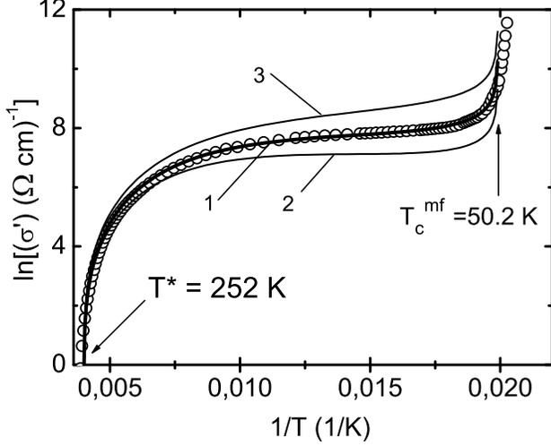
FIG. 8:  $\ln\sigma'$  vs  $1/T$  (circles) plotted in the whole temperature range from  $T^*$  down to  $T_c^{mf}$  at  $P=0$ . The solid curves are fits to the data with Eq. (10). The best fit is obtained when Eq. (10) is calculated for  $\Delta^*(T_c)=122.1$  K ( $D^* = 2\Delta^*(T_c^{mf})/k_B T_c = 5.0$  (curve 1)). Curves 2 and 3 corresponds to  $D^*=6$  and 4, respectively.
