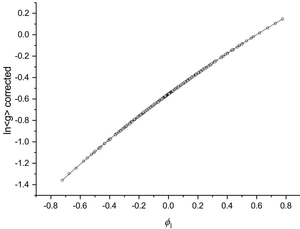
**Fig. B-2.** Demonstration of single parameter scaling for the conductance data. As explained in the text, the correction due to the irrelevant scaling variable has been subtracted from the simulation data. The solid line is  $F(\phi_1, 0)$
