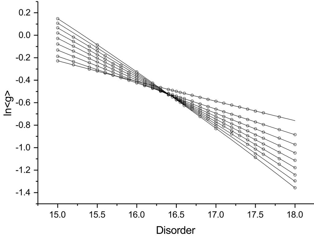
**Fig. B-1.** Finite size scaling fit (solids lines) to conductance data (circles) for Anderson's model of localisation in three dimensions. The errors of the data points are smaller than the symbol size.
