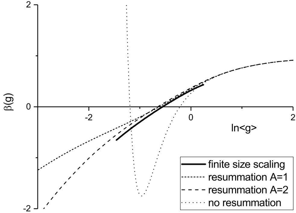
**Fig. 1.** Comparison of various approximations for the  $\beta$ -function for the  $d = 3$  orthogonal universality class with the  $\beta$ -function determined from finite size scaling (FSS) of numerical data obtained in simulations of Anderson's model of localisation. Plotting of the FSS result is restricted to the conductance range for which numerical data is available.
