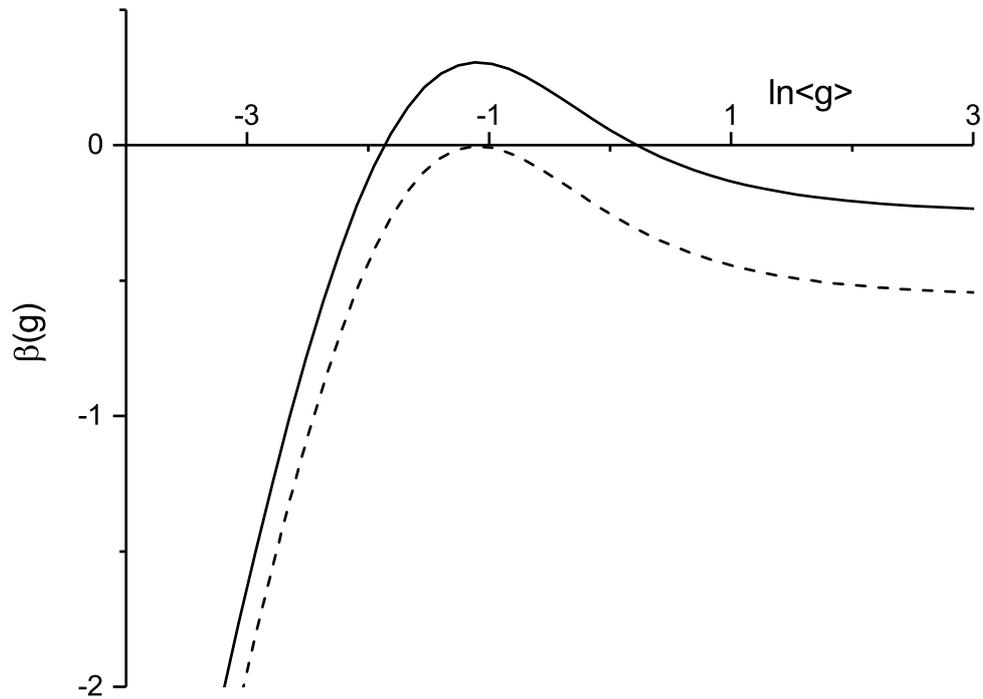
**Fig. 4.** The approximation for the  $\beta$  function for the symplectic symmetry class for  $d = 1.75$  (solid line) and  $d = 1.44$  (dashed line).
