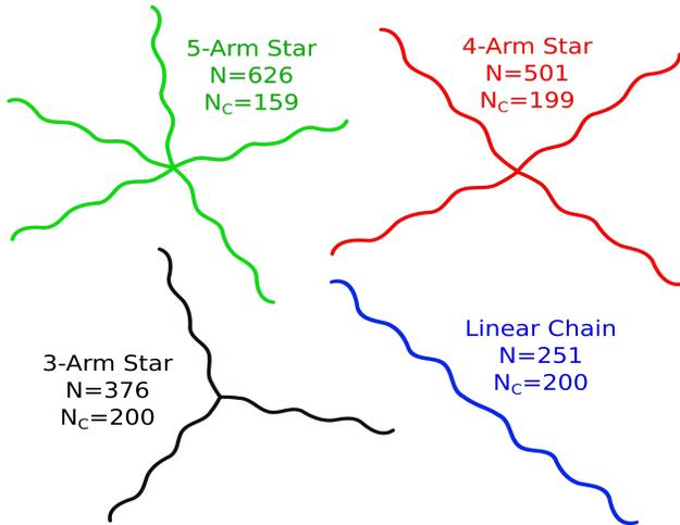
Figure 1: Schematic representation of the simulated systems.  $N_C$  is the number of polymers in the simulated box.  $N$  is the number of beads per polymer. Each arm is 125 beads long (corresponding to  $Z_a \approx 5$  entanglements).
