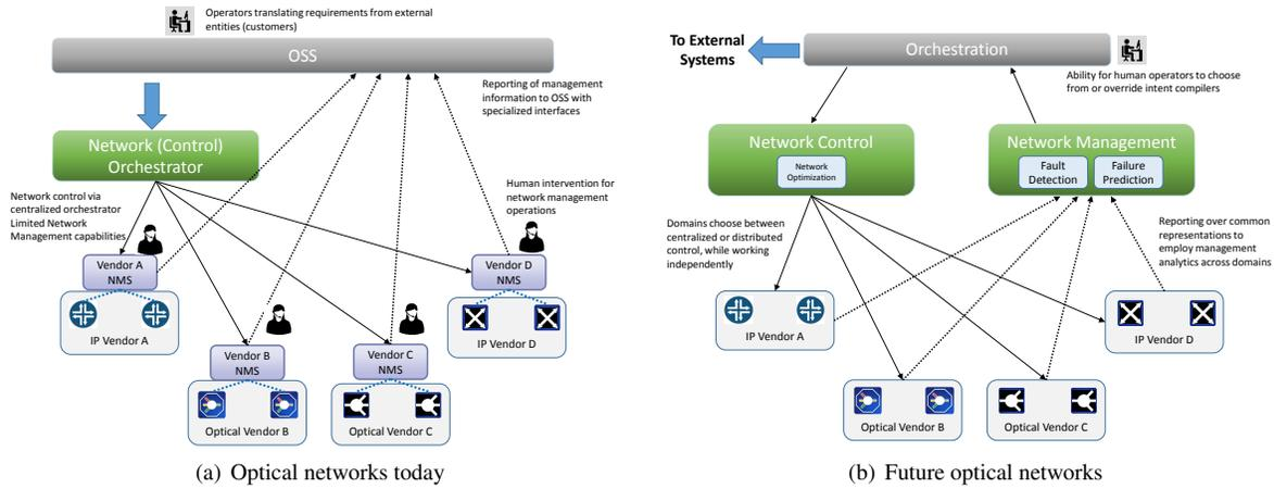
Fig. 1. Evolution of optical networking towards AI-based cognitive network and management.
