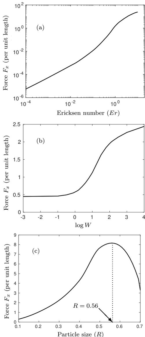
FIG. 6. The axial force  $F_x$  experienced on a static particle as a function of the (a) Ericksen number ( $Er$ ); (b) particle surface anchoring strength ( $\log W$ ); and (c) particle size ( $R$ ). The reference values of the parameters are  $R = 0.3$ ,  $Er = 1$  and  $\log W = 3$ . The values for all other parameters used for the calculation are given in Table I.
