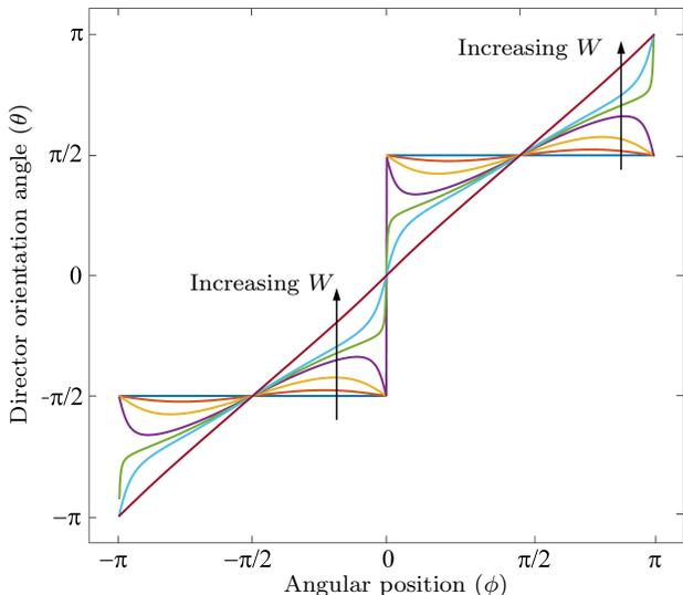
FIG. 3. Variation of the director angle on the particle surface with angular location as the anchoring strength is increased with  $\log W = -3, 0, 0.5, 0.8, 0.9, 1$  and  $2$ , with zero flow field ( $Er = 0$ ) for  $R = 0.3$ . The particle is located at the centre of the channel with homeotropic boundary conditions. The values taken for all other parameters used for the calculation are given in Table I.
