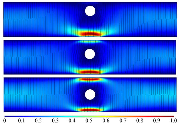
FIG. 7. Snapshots showing the time evolution of a particle placed inside a NLC microchannel with initial position  $Y = 0.5$  as it relaxes towards the centre: (a)  $T = 0$ ; (b)  $T = 12.5$ ; and (c)  $T = 100$ . Here  $R = 0.3$  and  $Er = 0.02$ . The anchoring conditions on the particle and channel walls are homeotropic. The values for all other parameters used for the calculation are given in Table I.
