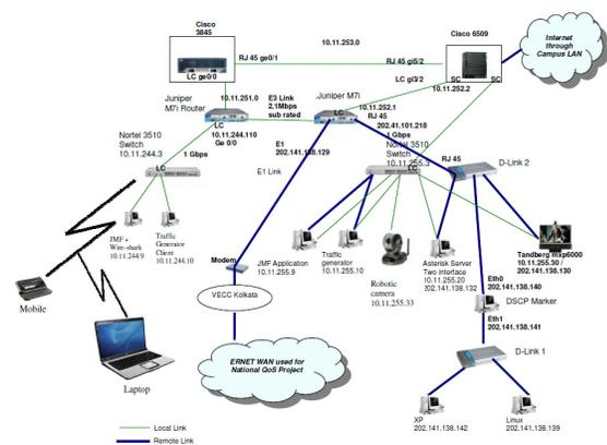
Fig. 1: Wireless IP QoS testbed
