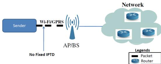
Fig. 4: No fixed Inter Packet Transmission Delay
