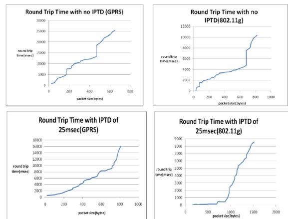
Fig. 9: RTT comparison for Wi-Fi and GPRS for various IPTD
