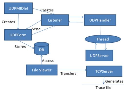
Fig. 3: Test tool architecture
