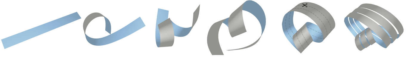
Fig. 21. Our local isometry model allows us to deform, glue, and cut a surface while maintaining an exact discrete notion of isometry. In this figure we twist a long strip twice, glue it, and then cut it along two horizontal sections, creating three interleaved knotted surfaces.
