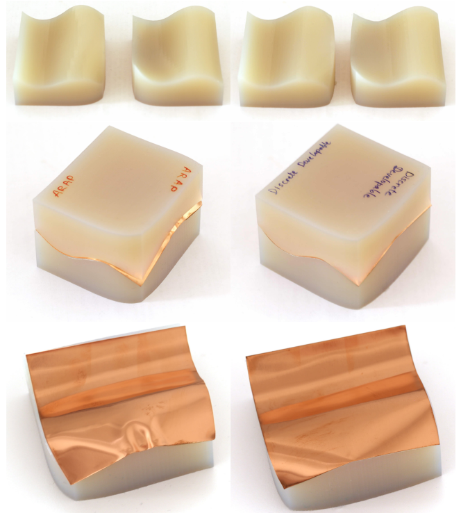
Fig. 14. Validation by fabrication. We 3D-printed a “sandwich” (top row) whose inner cut surface is the result of deforming a flat square using ARAP (left column) and our editing system for discrete developable surfaces (right column) using the same (soft) positional constraints. We cut two squares out of a thin copper sheet with the dimensions of the initial model before deformation, and we sandwiched these squares in the fabricated pieces (second row). Not surprisingly, since the ARAP result is not developable, the sheet wrinkles and buckles (bottom left), while our result exhibits pure bending (bottom right). Note that our result is smooth everywhere except at the boundary, where a cone-like kink is created in the digital model to remedy the doubly curved ARAP surface.
