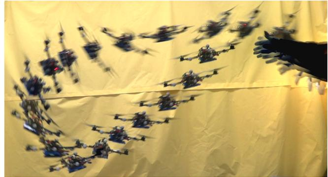
Figure 1: The quadrotor stabilizes from a hand throw. The motor was enabled after it left the hand
