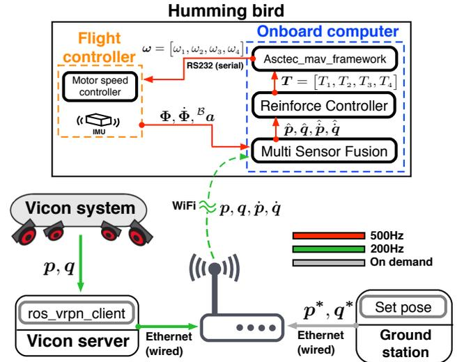
Figure 6: System diagram used for the experiments. Different colors denote the corresponding rate respectively.  $p, q, \dot{p}, \dot{q}$  are position, orientation and their velocities.  $p^*$  and  $\hat{p}$  denote the desired goal and estimated position.  $T$  and  $\omega$  are thrust in N and rotor speed in rad/s.  $\Phi, \dot{\Phi}, {}^B a$  represent IMU measurements; orientation, angular velocity, and linear acceleration in body frame.
