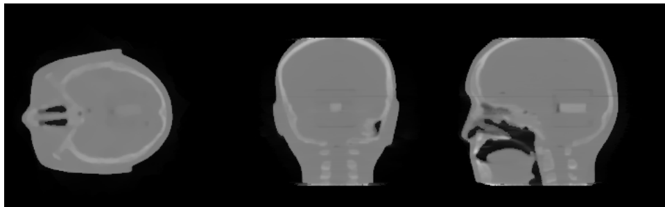
Fig. 5. Transverse (left), coronal (middle), and sagittal (right) slices of pCT reconstruction of pediatric head phantom (CIRS customized Model 715HN).
