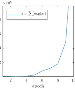
Figure 5: Magnitude of the softmax normalization term,  $s = \sum_i e^{x_i}$ , recorded for a 10-layer CNN trained on CIFAR-10. It starts out with  $s = 2,342$  and blows up from there.
