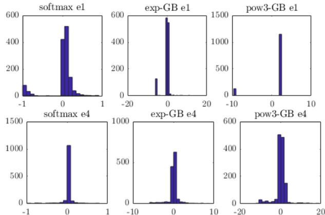
Figure 2: **Top:** The distribution of output layer error gradients for softmax, linear with exponential boosting, and linear with cubic boosting at the start of epoch 1; training a 10-layer CNN on CIFAR-10. **Bottom:** same, but for epoch 4.
