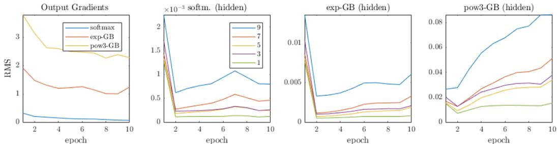
Figure 3: RMS of error gradients over ten epochs of training a 10-layer CNN on CIFAR-10. **Left:** output layer. **Rest:** every second hidden layer. Note the upwards trend from epoch 2 onwards in the hidden layers for GB.
