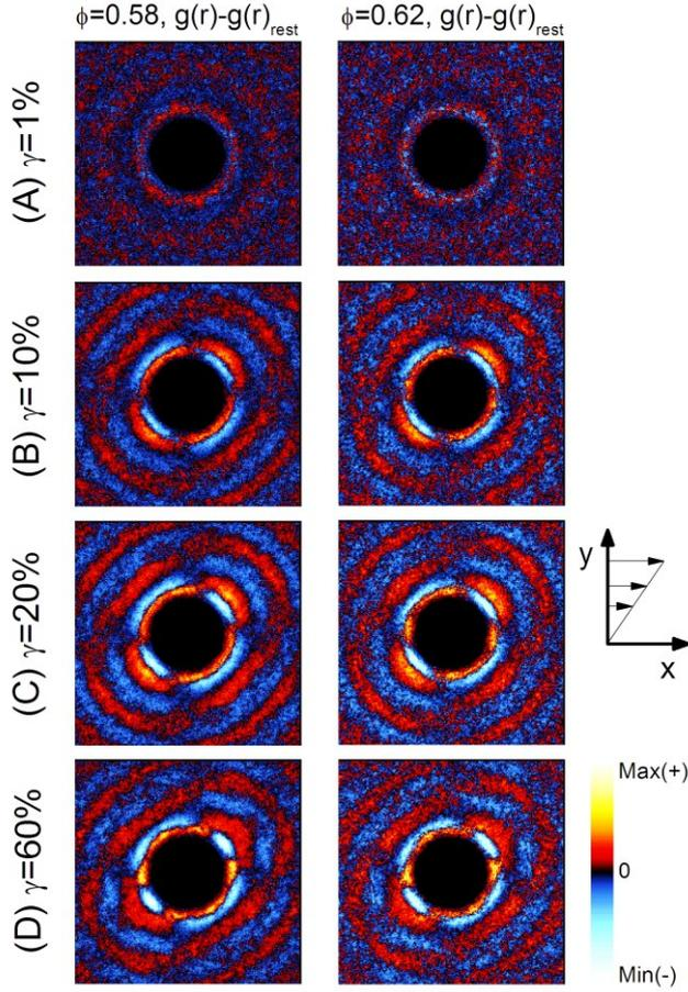
FIG. 10: Pair distribution function  $g(r)$  in the velocity-gradient ( $xy$ ) plane after subtraction of the state at rest for  $\phi=0.58$  (left) and  $\phi=0.62$  (right) for  $Pe=1$  at strains of 1%, 10%, 20% and 60%, from top to bottom, corresponding to the A, B, C and D positions in Fig. 11. The  $g(r)$  have been normalized with the same factor for all strains and  $\phi$ .
