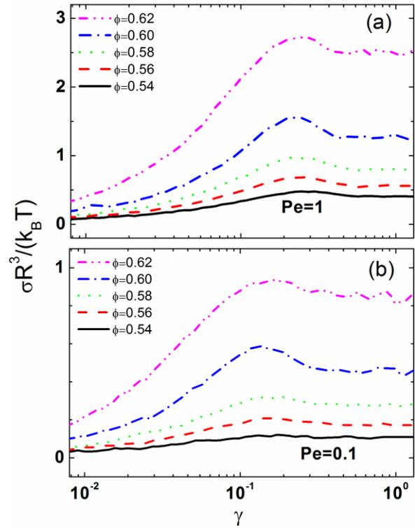
FIG. 7: Scaled stress,  $\sigma R^3 / K_B T$ , versus strain,  $\gamma$ , in a lin-log plot from step rate start-up BD simulations for two different rates (a)  $Pe=1$  and (b)  $Pe=0.1$  at various  $\phi$  as indicated in the legend.
