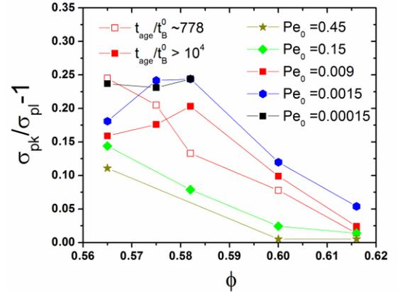
FIG. 6: Magnitude of the stress overshoot  $\sigma_{pk}/\sigma_{pl}-1$  as a function of volume fraction  $\phi$  (for the PMMA particles with  $R=183$  nm in octadecene/bromonaphthalene) at different shear rates quantified by the Peclet number  $Pe_0$  (as indicated) in the limit of long ageing time (here for  $t/t_B^0 \geq 10^4$ ). In addition for an intermediate  $Pe_0$
