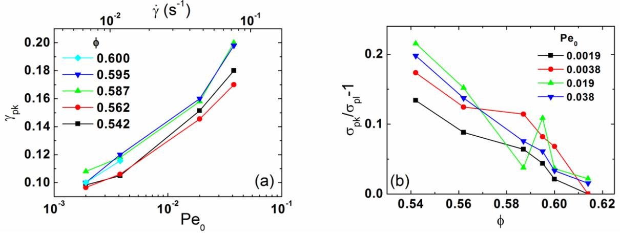
FIG. 4: Data from step rate experiments for the R=267 nm PMMA particles in decalin at an ageing time of 200s ( $t/t_B^0 \approx 667$ ): (a) strain values of the peaks  $\sigma_{pk}$  as seen in the Figs. 2 and 3 plotted against  $Pe_0$  for different  $\phi$ . (b) The normalized magnitude of the stress peak,  $\sigma_{pk}/\sigma_{pl}-1$ , plotted against  $\phi$  for various rates indicating the loss of the peak at high  $\phi$ .
