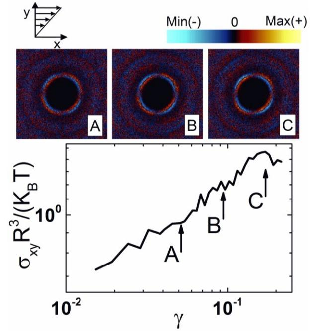
FIG. 14: Above: Pair distribution function  $g(r)$  in the velocity-gradient ( $xy$ ) plane after subtraction of the state at rest for confocal measurements at  $\phi=0.56$  for  $Pe_{sc}=0.594$  at strains of 5%, 9% and 17% corresponding to the A, B and C positions as shown in the below. Below: The stress calculated based on confocal micrographs as described in the text.
