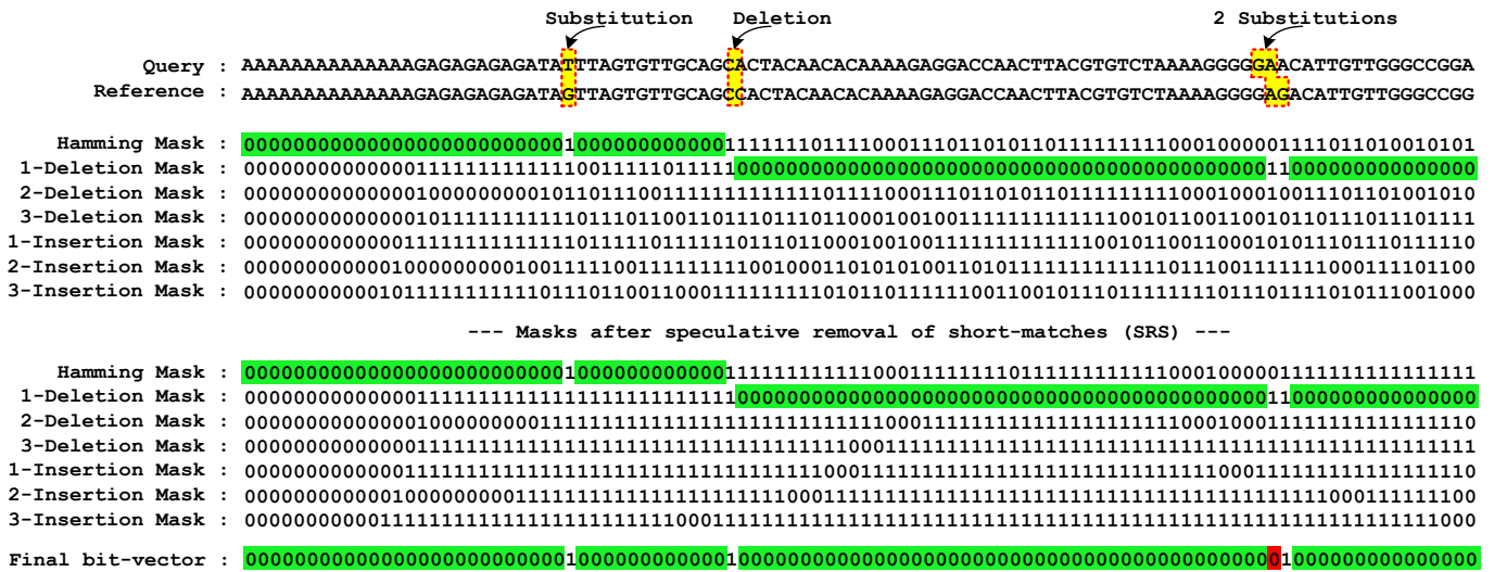
Fig. 2: An example of an alignment with all its generated masks, where the edit distance threshold ( E ) is set to 3. The green highlighted subsequences are part of the correct alignment. The red highlighted bit in the final bit-vector is a wrong alignment provided by SHD. The correct alignment (highlighted in yellow) shows that there are three substitutions and a single deletion, while SHD detects only two substitutions and a single deletion.
