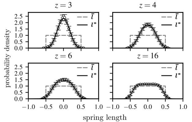
FIG. 4. Probability density  $p_{l^*}(\ell^*)$  for the final spring lengths for networks with  $N = 1000$  and varying  $z$ . Solid black lines show the analytic expression for  $p_{l^*}(\ell^*)$  [16]; data points correspond to averages over 50 simulations. The error bars correspond to the standard deviation. For comparison, we show the initial uniform spring length distribution  $p_{\bar{l}}(\bar{\ell})$  as a gray dashed line.
