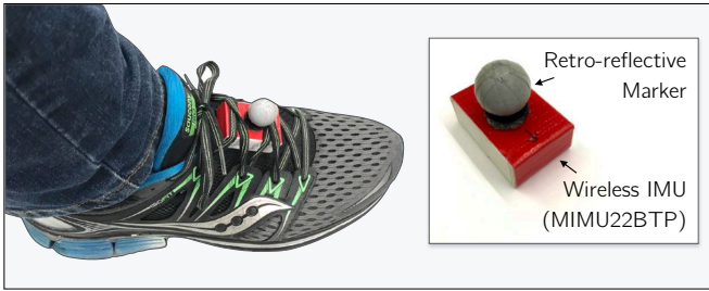
Fig. 3: Our apparatus: an Inertial Elements MIMU22BTP(X) [17] wireless 4-IMU array mounted to the foot of a test subject. Note that we use both the MIMU22BTP and its X variant (which has a larger lithium-ion battery but identical sensing hardware).
