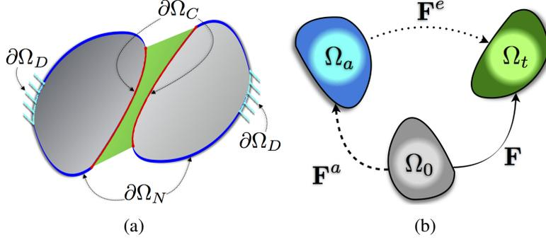
Figure 1: Schematic representation of (a) imposed boundary conditions, e. g., Dirichlet,  $\partial\Omega_D$ , Neumann,  $\partial\Omega_N$ , and Contact,  $\partial\Omega_C$ ; (b) multiplicative decomposition of the deformation gradient in total  $\mathbf{F}$ , active,  $\mathbf{F}_a$ , and elastic,  $\mathbf{F}_e$ , maps associated with the reference,  $\Omega_0$ , active,  $\Omega_a$ , and current,  $\Omega_t$ , configurations.
