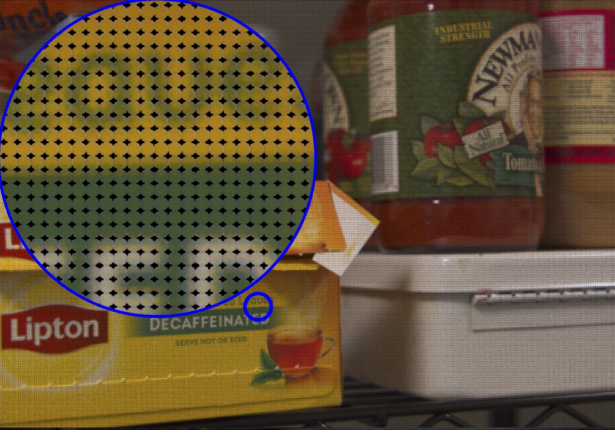
Fig. 2: Light field captured by a Lytro Illum camera. A zoomed-in region is overlaid to show the individual lenslet regions.
