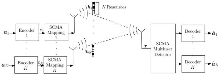
Fig. 1. The system model for uplink transmission of a coded SCMA system with  $K$  users multiplexed over  $N$  resources with an overloading factor of  $K/N$ .
