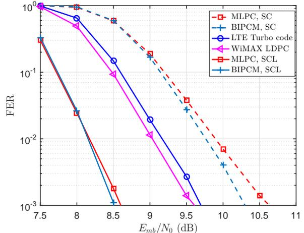
Fig. 4. The comparison among an SC-decoded MLPC system, an SC-decoded BIPCM system, both with  $N_c = 2048$ , LTE turbo coded system with  $N_c = 2070$ , WiMAX LDPC system with  $N_c = 2016$ , an SCL-decoded MLPC system, and an SCL-decoded BIPCM system, both with  $N_c = 2048$ . The overall code rate for all cases is  $R = 2/3$ . All systems operate in fast fading.
