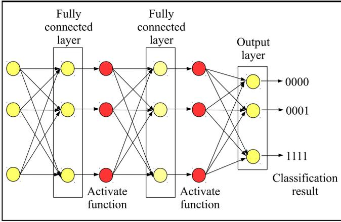
Fig. 4. Multiple layer perceptron (MLP).
