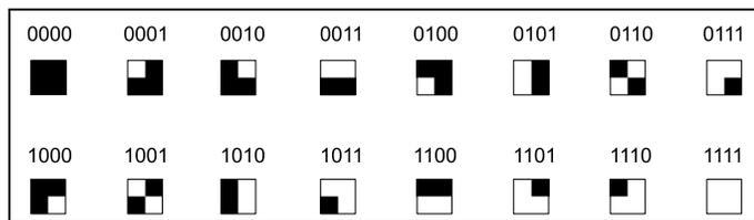
Fig. 2. 4-bit representation using 16 fragments.
