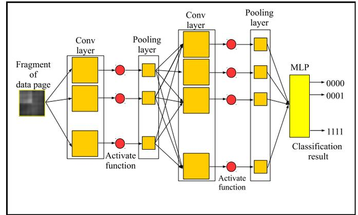
Fig. 3. Deep-learning-based classification for holographic memory.
