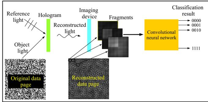
Fig. 1. Deep learning-based classification for holographic memory.
