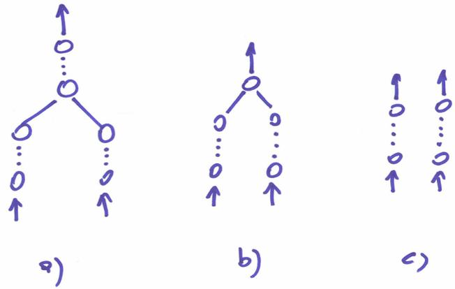
Fig. 2. The proposed methods use network architectures of varying complexity: a) convolutional branches and fc connection layers (YCNN, GOTURN), b) convolutional branches and a single connection layer (SiamFC, CFNet), c) convolutional branches with equal final normalisation layers (SINT).
