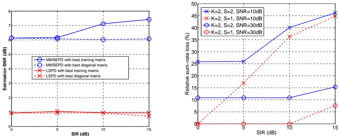
(a) Scenario:  $K = 2$ ,  $S = 1$ , and  $\text{SNR}(\text{dB}) = 30$ ,  $\epsilon = 0$ ,  $N = 2$  quantization bits. Using a diagonal training matrix typically induces a small performance loss in terms of ESNR even in worst-case scenarios.
