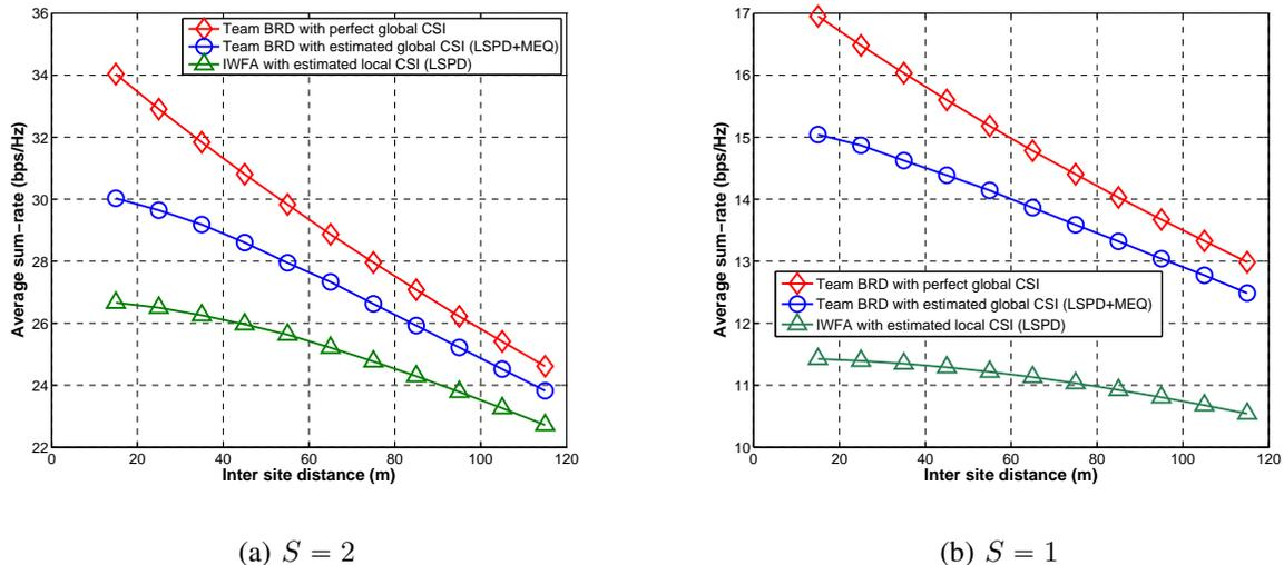
Fig. 4: The above curves are obtained in the scenario of Fig. 4 in which  $K = 9$  transmitter-receiver pairs,  $\text{SNR}(\text{dB}) = 30$ , the FCSE is given by  $\epsilon = 0.01$ ,  $N = 8$  quantization bits for the RSSI, and  $L = 2$  power levels. Using the most simple estimation schemes proposed in this paper namely LSPD and MEQ can bridge the gap between the IWFA and the team BRD with perfect CSI, about 50% when  $S = 2$  and about 65% when  $S = 1$ .
