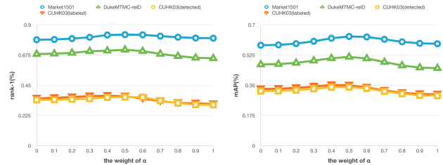
Fig. 5 Sensitivity of person re-ID accuracy to parameter \alpha . Rank-1 accuracy(%) and mAP(%) on three datasets are shown.
