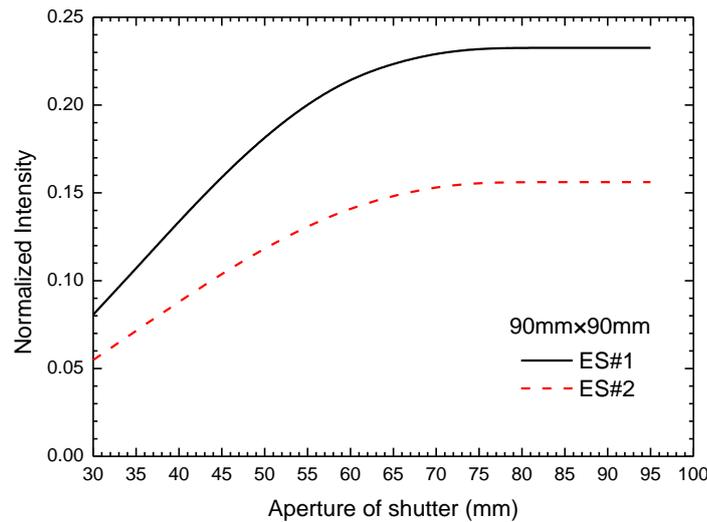
**Fig. 7 Neutron intensities of two endstations vs. shutter aperture by fixing the apertures of Collimator 1 & 2 (76 mm & 90 mm, respectively).**
