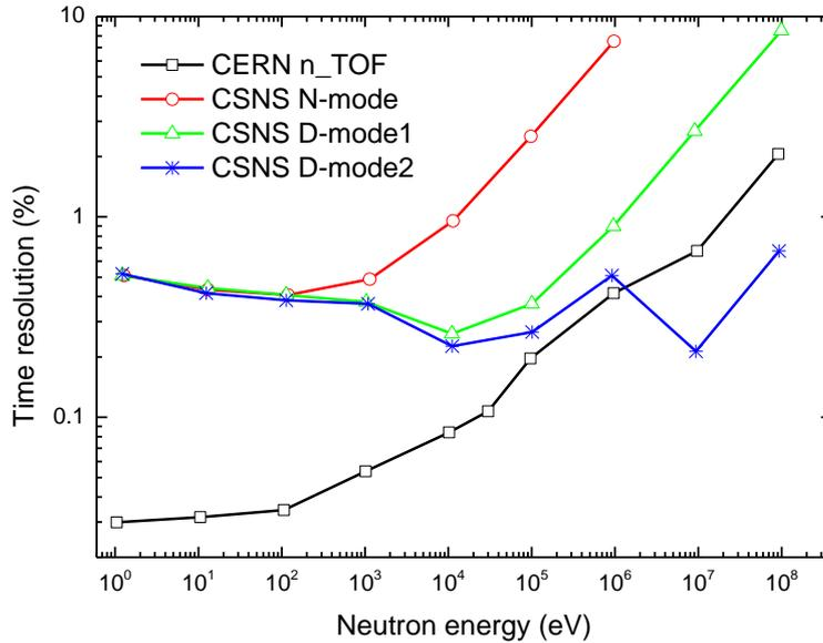
**Fig. 3 Time resolution comparison between CERN n-TOF and CSNS Back-n on different modes at 80 m**
