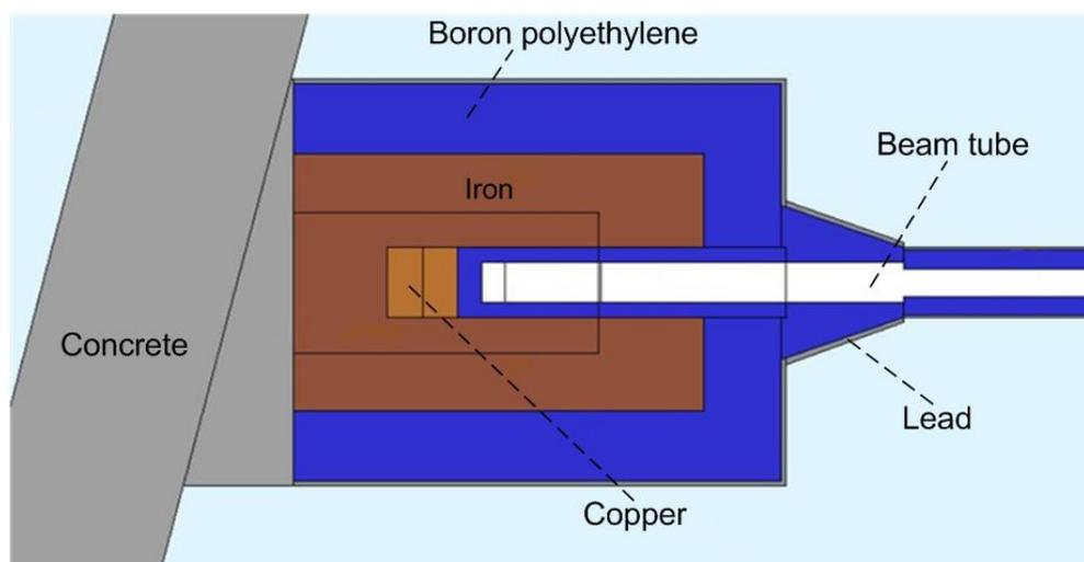
Fig. 14 Geometry structure of the neutron dump.
