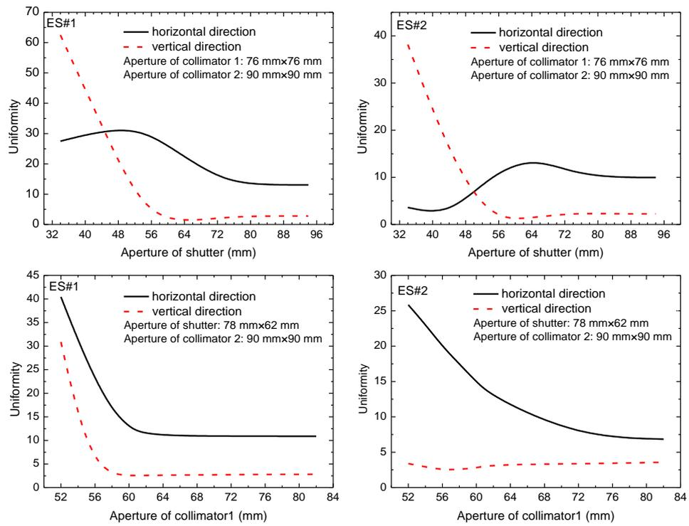
**Fig. 8. Neutron beam-spot uniformity for 90 mm × 90 mm beam spot in the horizontal and vertical directions in ES#1 & ES#2 vs. apertures of shutter and collimator.**
