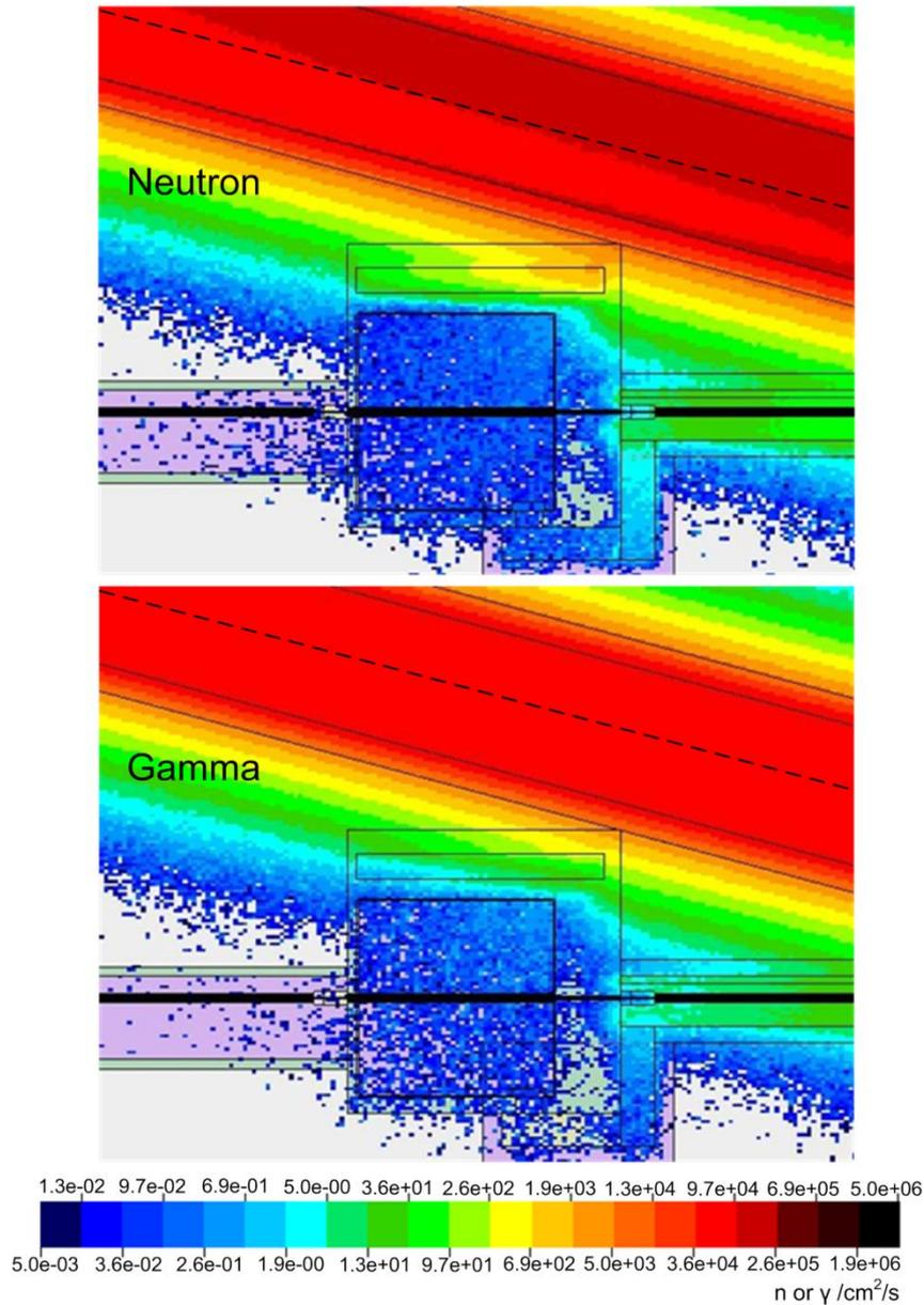
**Fig. 10 Neutron & gamma backgrounds in the ES#1 experimental hall. The dotted line represents the line-type proton loss source.**
