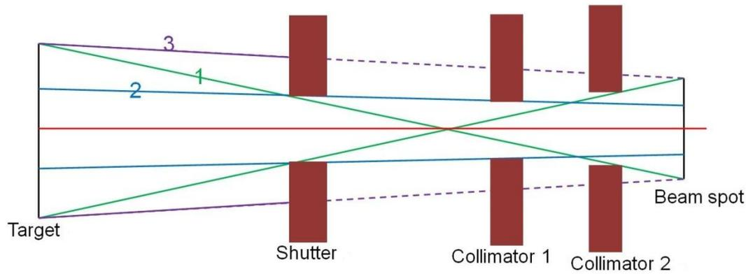
**Fig. 6 A simplified depiction of the neutron beam optics**
