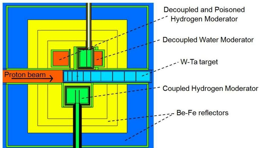
**Fig. 1 Geometry of target-moderator-reflector (TMR) model**
