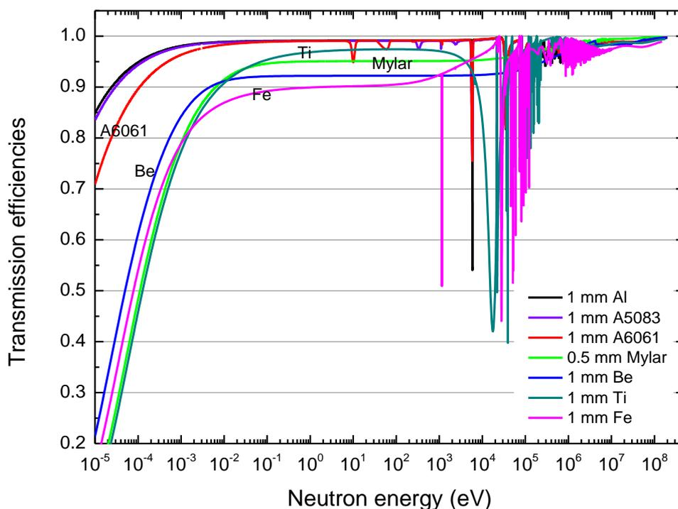
**Fig. 13 Comparison of the transmission efficiencies for different materials in the whole neutron energy range**
