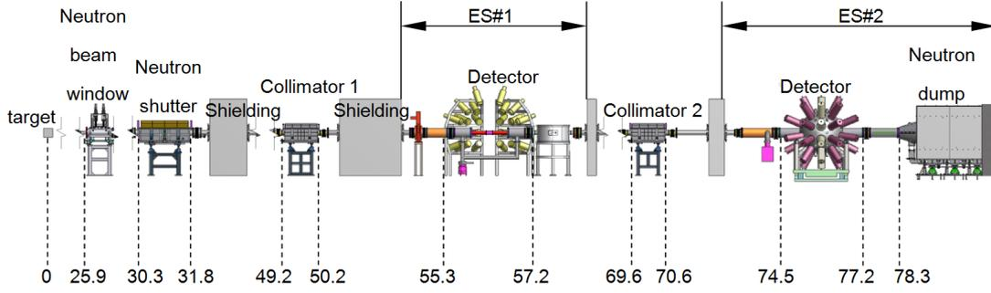
**Fig. 4. Layout of the Back-n beam line from the spallation target to the beam dump (distances are given in meters).**
