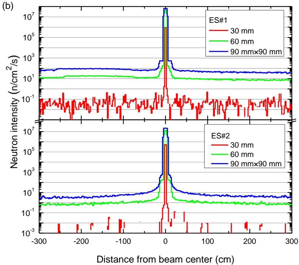
**Fig. 11 Neutron beams and backgrounds at 100 kW: (a) Neutron & gamma fluences (From up to down:  $\Phi$ 30 mm,  $\Phi$ 60 mm, 90 mm  $\times$  90 mm); (b) and neutron profiles at ES#1 and ES#2**
