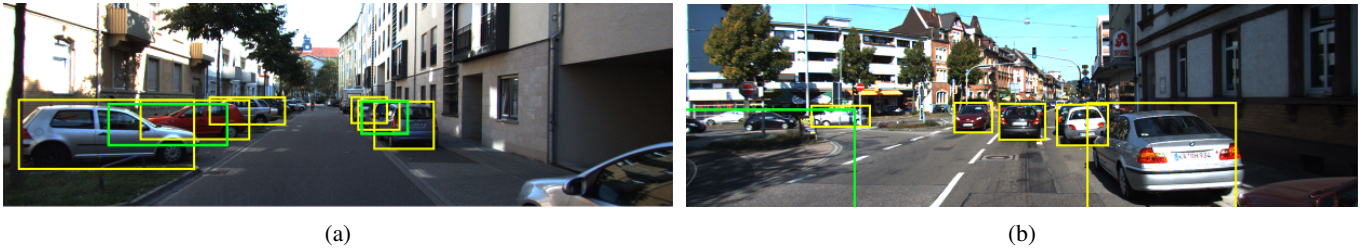
Fig. 2: (a) In crowded regions, multi-object tracker creates some duplicates tracks that straddle multiple cars (shown in green). (b) Region based tracker maintains track even after car exits the scene (shown in green)
