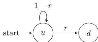
Figure 3: The drop clock, a Markov chain with a probability  $r$  to permanently transition to state  $d$  and remain there.
