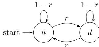
Figure 1: The alternator clock. It switches one state to the other with probability  $r$ .
