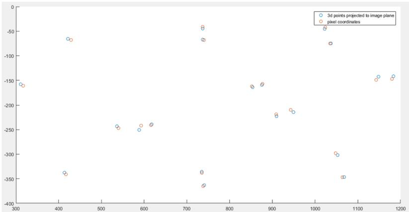
**Fig. 4.** Back-projected 3D points and 2D points on the image plane (in pixels) using E-PnP. The 20 points (refer to table 1) seem to be aligned, however, the transformation obtained deviates from the measured values.
