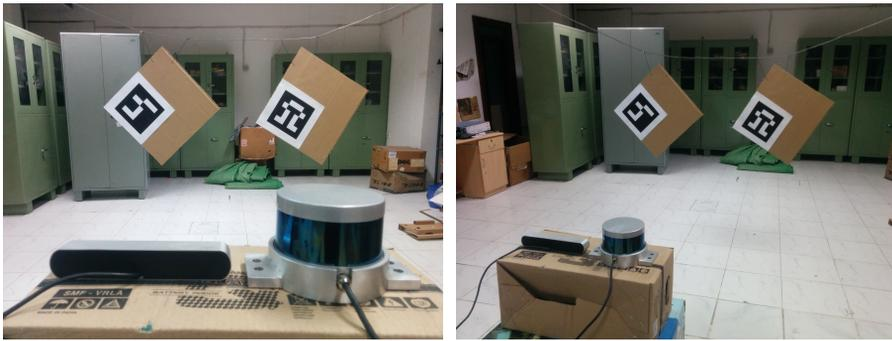
**Fig. 6.** Experimental setup with rectangular cardboard and ArUco markers using 3D-3D correspondences.
