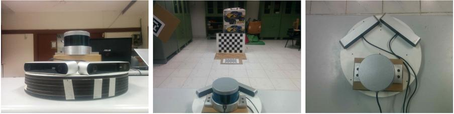
**Fig. 12.** Experimental setup with cameras kept at about 80 degrees. The calibration for such configuration shows that our unique method can be, in principle, used for extrinsically calibrating cameras with no field-of-view overlap.
