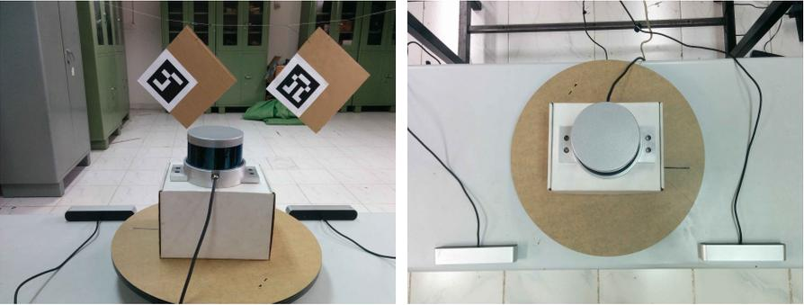
**Fig. 11.** Experimental setup for comparing point cloud fusion when using manual measurement versus using transformation obtained from `lidar_camera_calibration`.
