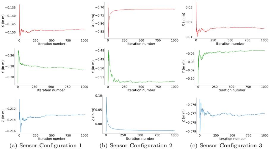
**Fig. 9.** At the  $i$ -th iteration, the plots show the translation values after averaging estimates from the previous  $i$ -iterations. The plots are show translation in  $X, Y, Z$  when the LiDAR and camera were kept in three random configurations(positions).
