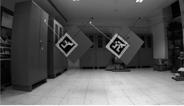
**Fig. 8.** Rotation and translation between the board's frame-of-reference and the camera's frame-of-reference are found using the ArUco markers. This transformation is used to transform the 3D corner points from the board frame to the camera frame.
