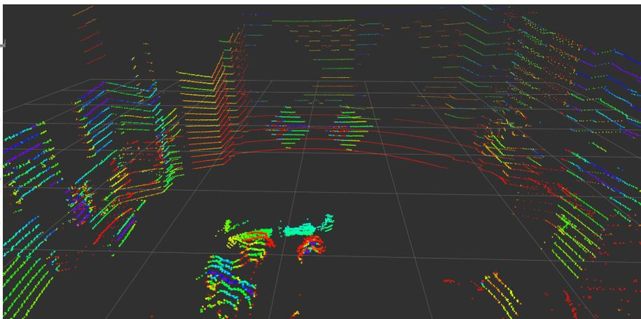
**Fig. 1.** LiDAR scan of the experimental setup. 3D point correspondences are obtained in the LiDAR as well as camera frame. The two sets of 3D points are used to solve for a rotation and then a translation.
