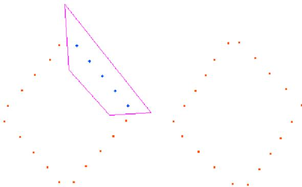
**Fig. 3.** Marking line segments in the 3D-pointcloud. The ROS node allows for manually marking segments by drawing polygons around each line segment and also calculate their intersections.
