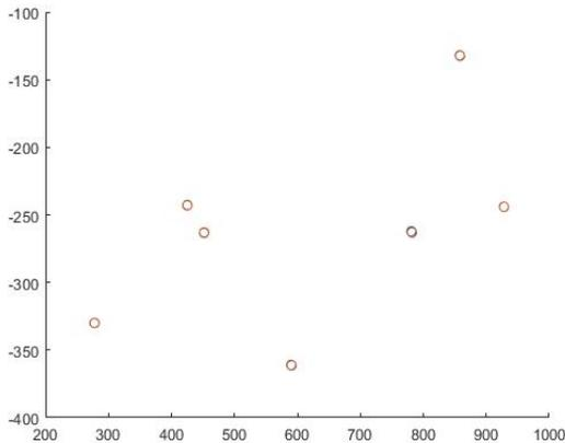
**Fig. 5.** Projection of 3D inlier points(after applying  $[R|t]$  from RanSaC E-PnP) and corresponding 2D points on *rot\_data*. The projected 3D and 2D points align very well but again, there is deviation from the manually measured values (refer to table 3).
