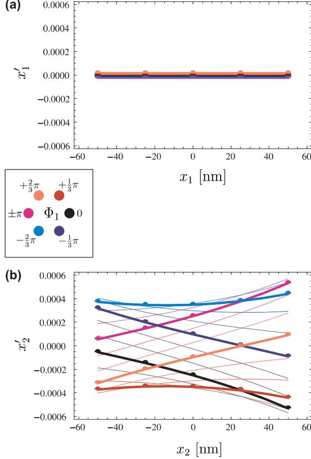
FIG. 4. The properties of the transfer function for the unit cell shown in Fig. 3. (a) Assumed  $(x_1, x'_1)$  at the entrance of the cell. (b) Calculated  $(x_2, x'_2)$  at the exit of the cell. The result depends on the initial phase  $\Phi_1$  (color coded). The thicker lines correspond to six selected phases:  $-\pi, -\frac{2}{3}\pi, -\frac{1}{3}\pi, 0, \frac{1}{3}\pi, \frac{2}{3}\pi$ .
