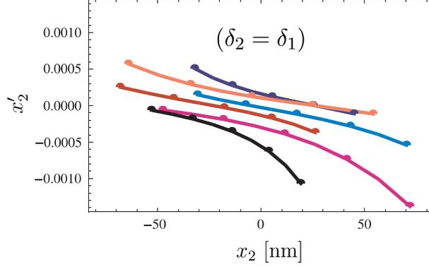
FIG. 10. The focusing properties of the  $\mathcal{O}_{5+1/2}\overline{\mathcal{R}}^8\mathcal{O}_{5+1/2}\overline{\mathcal{R}}^8$  segment calculated using „spoiled” ( $\delta_2 = \delta_1$ ) transfer function (compare with the correct result in Fig. 7(c)).
