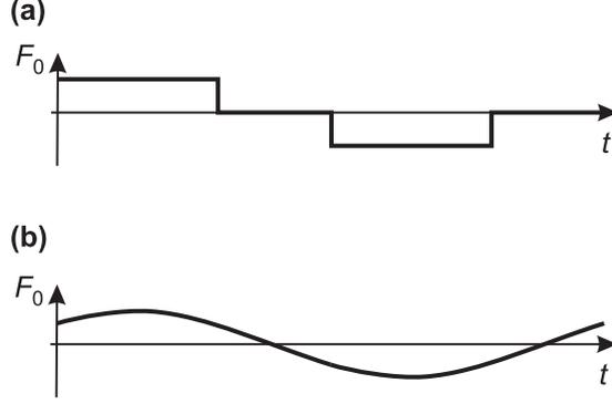
FIG. 11. (a) Time dependence of the focusing force in a FODO-like DLA cell (Fig. 6). (b) Harmonic oscillation leading to classical ponderomotive force.
