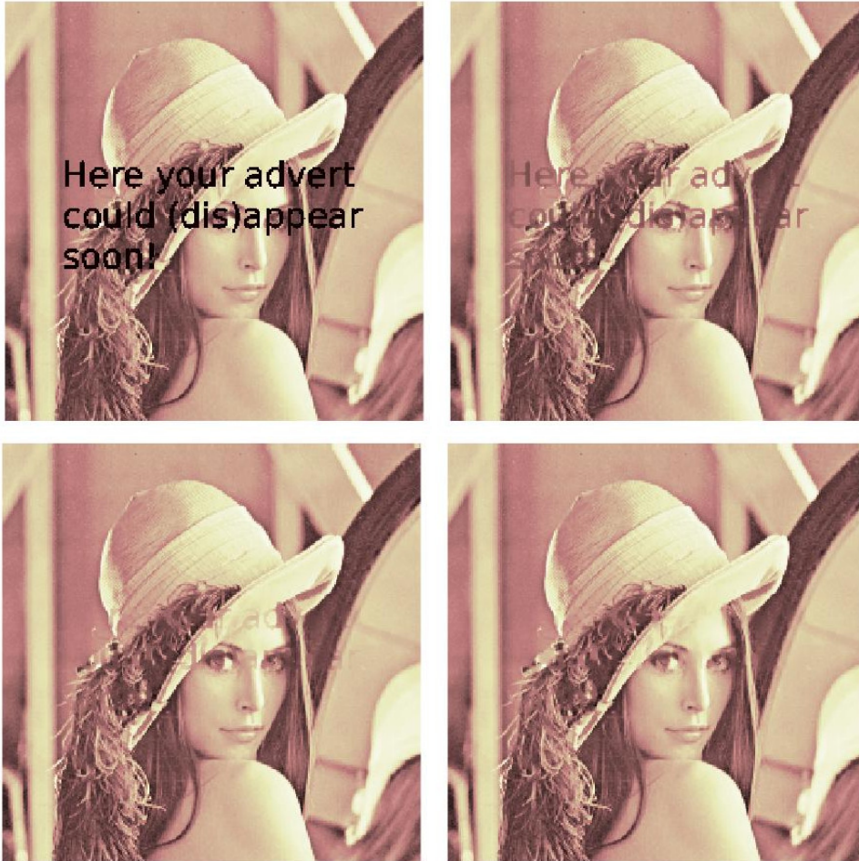
FIG. 8. Removing text from Lena: text image (top, left), spline inpainting using order 3 (top, right), order 4 (bottom, left) and 5 (bottom, right). Obtained SNR values: 23.2, 28.45 and 31.25.
