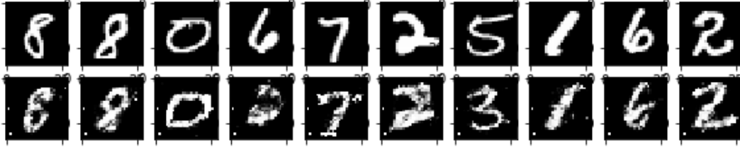
Figure 4: VEEGAN method can be used like ALI to perform inference. The means output from the reconstructor network for the real images in the top row are used as the latent features to samples the generated images in the bottom row.
