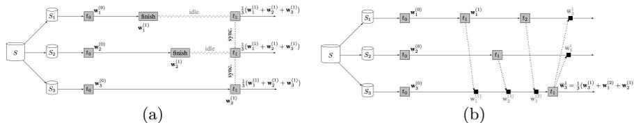
Fig. 1: Diagrams of the distributed synchronous (a) and asynchronous (b) frameworks.
